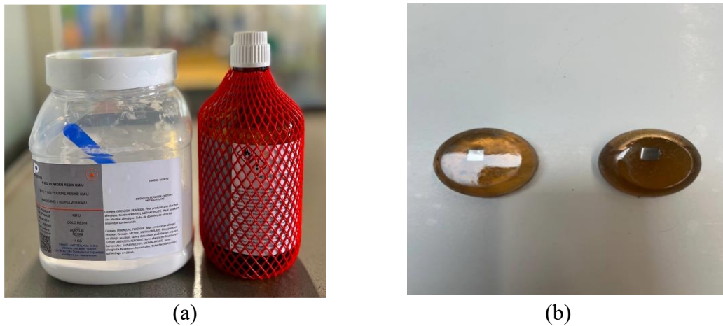
Fig. 30. Sample mounting procedure (a) Specimens were embedded in acrylic resin using a methyl methacrylate hardener to ensure structural stability and ease of handling during subsequent metallographic preparation. (b) After curing, the mounted samples were extracted from the mould and prepared for sequential grinding and polishing.
