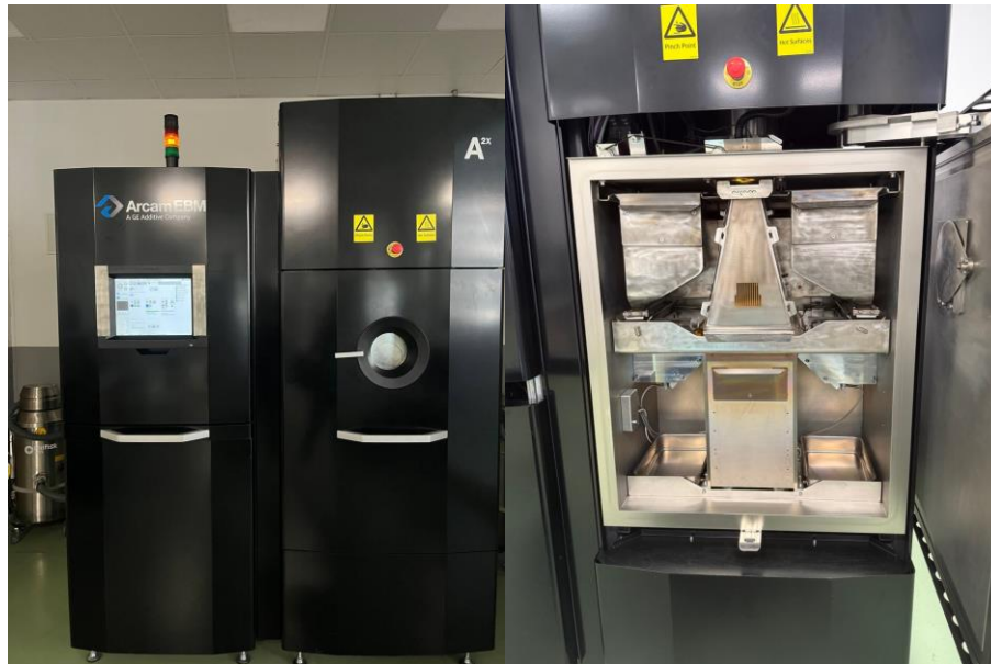
Fig. 28. Arcam A2X Electron Beam Powder Bed Fusion system employed in this study for Ti-6Al-4V –Cu fabrication.
