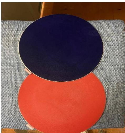
Fig. 32. Polishing media used for final surface preparation. Polishing was carried out using multi-stage polishing pads with 3 \mu\text{m} (blue) and 1 \mu\text{m} (pink) grit sizes to progressively eliminate residual surface deformation and achieve a deformation-free surface suitable for high-resolution microstructural characterization.
