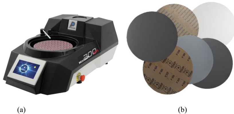
Fig. 31. Grinding setup and abrasive sequence, (a) Metallographic grinding and polishing were performed using a Presi automatic preparation system to ensure controlled and reproducible surface finishing. (b) A progressive abrasive sequence (P480, P600, P800, P1200, and P2400) was applied to systematically reduce surface roughness and remove deformation induced during sectioning.
