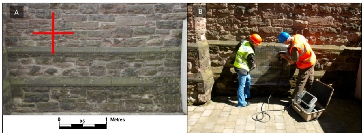
Figure 3. (A) Location of the perpendicular test lines, marked in red, on the study wall surface. (B) operation of the equipment on the study wall section (Johnston et al., 2018)
