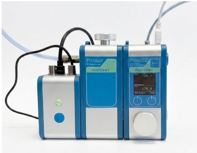
Figure 3.1 Fluigent LineUp microfluidic control system used for pressure-driven flow characterization.
