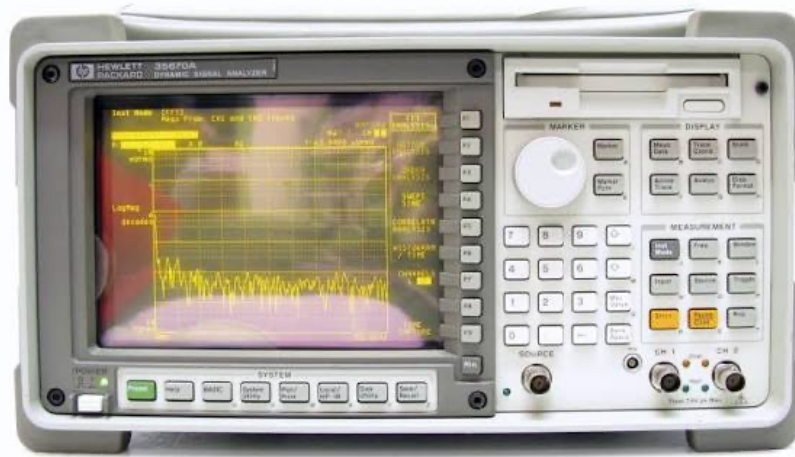
Figure 3.9 HP35670A Dynamic Signal Analyzer [37] used for resonance frequency measurements of the Coriolis microsensor.
