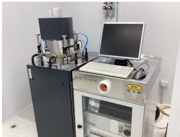
Figure 2.16 EVG 510 thermocompression bonding system.
