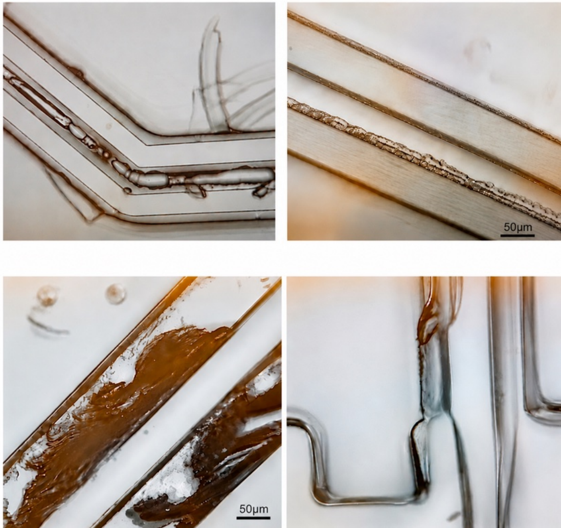
Figure 2.25 Cracking and collapse of the microchannel walls following excessive thermomechanical loading.
