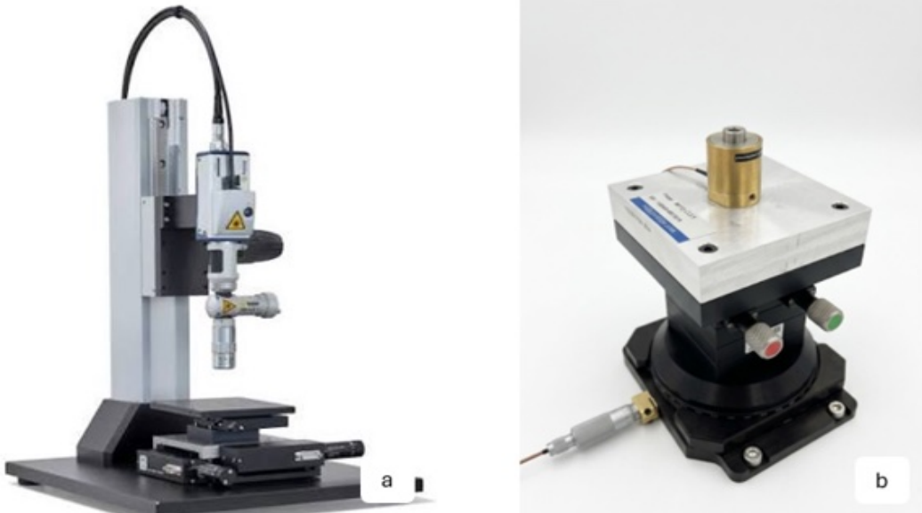
Figure 3.8 Experimental setup for dynamic characterization of the Coriolis microsensor: (a) LDV MSA-060 Micro System Analyzer employed for non-contact optical vibration measurements; (b) piezoelectric actuation system used for mechanical excitation of the \Omega -shaped microsensor.
