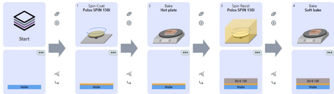
Figure 2.2 Sequence for the preparation of the first base layer of the device. Schematic prepared using FabuBlox.
