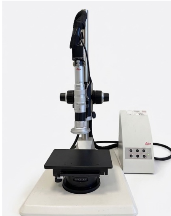
Figure 3.3 Leica Microsystems digital microscope used for real-time optical inspection of fluid flow within the \Omega -shaped microchannels.
