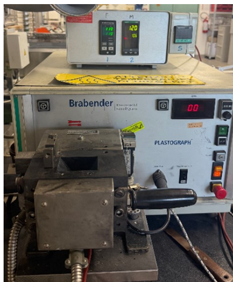
Fig. 9. Brabender Plastograph internal mixer used for compounding NR/SBR rubber composites.
