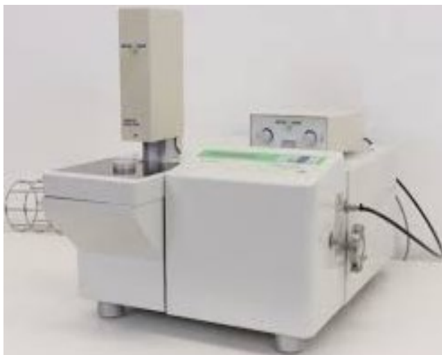
Fig. 13. TGA analyzer (Mettler Toledo TGA-SDTA 851) for thermal degradation profiling.
