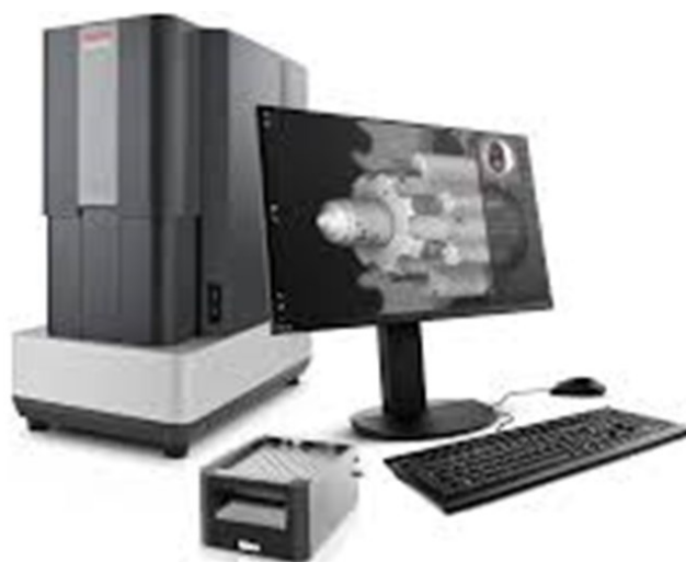
Fig. 11. SEM (Phenom XL) with EDS for surface morphology and elemental analysis.
