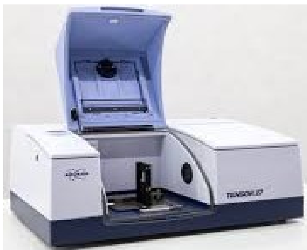
Fig. 12. FTIR spectrometer (Bruker TENSOR 27) for functional group identification.
