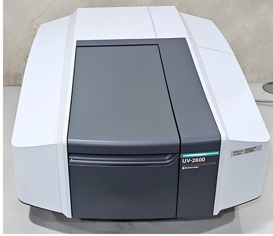
Figura 2.9: UV-2600 UV-Vis spectrophotometer (Shimadzu)
