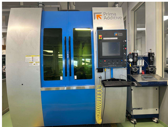
Figure 2.2-1 Prima Additive Laserdyne 430 DED machine
