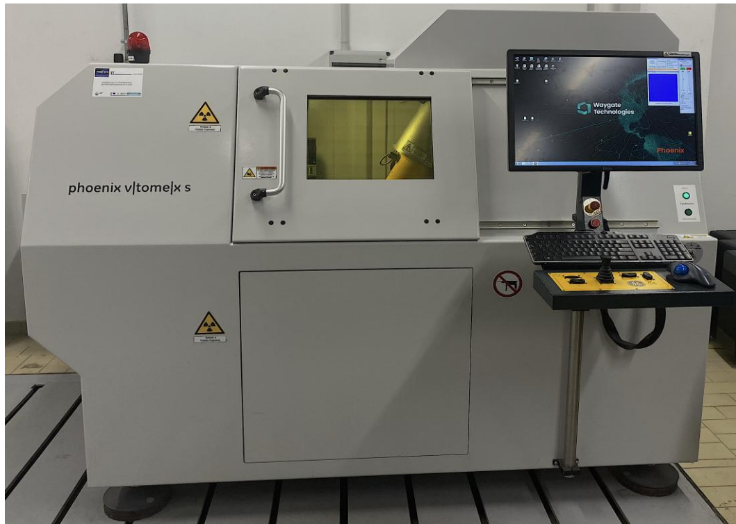
Figure 29. X-ray computed tomography system and sample holder used for three-dimensional defect characterization of LPBF Ti-5553 specimens.
