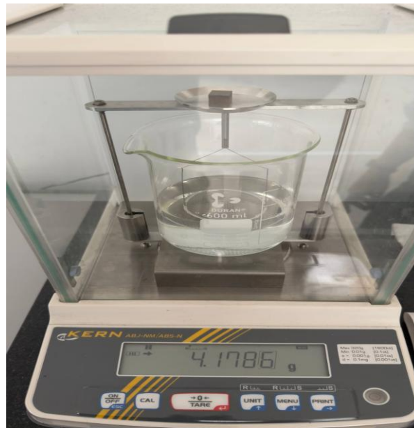
Figure 28. Archimedes density-measurement setup used for the as-built LPBF Ti-5553 cubic specimens before surface modification.
