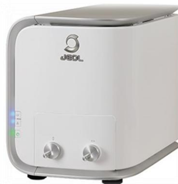
Figure 34. JEOL JCM-6000 Plus scanning electron microscope used for microstructural and defect characterization of the LPBF Ti-5553 specimens.
