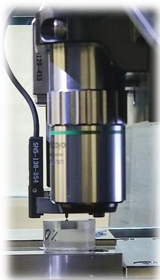
Figure 36. Hysitron TI 950 TriboIndenter used for nanoindentation testing of polished LPBF Ti-5553 specimens.
