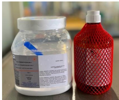
Figure 30. Mounting stage for metallographic preparation of LPBF Ti-5553 specimens, acrylic resin KMU and methyl methacrylate hardener used for mounting.
