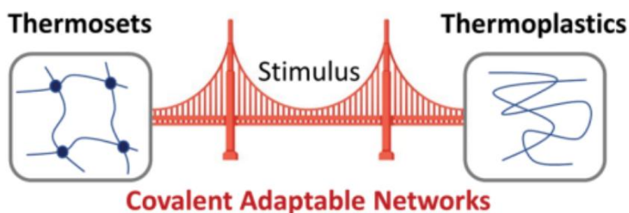
Figure 9 - Schematic illustration of the Covalent Adaptable Network (CAN) concept, combining the reprocessability of thermoplastics with the mechanical robustness of thermosets.
