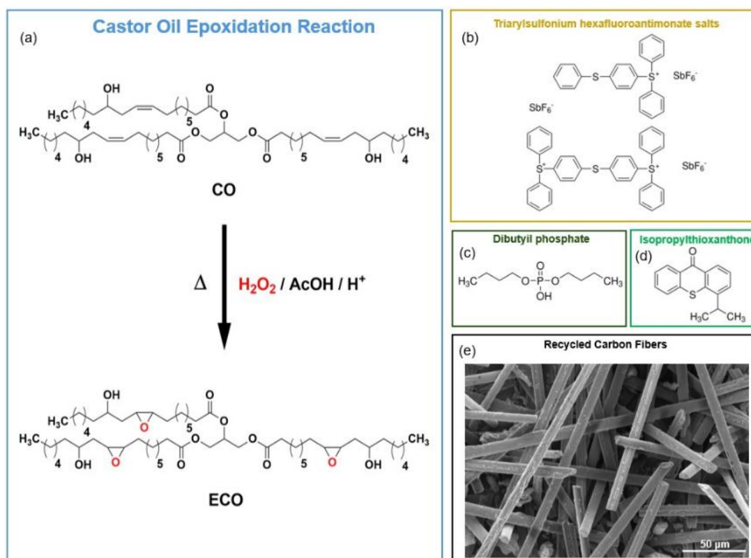
Figure 20 - Structural formulas of the components employed in the ECO-based formulation
