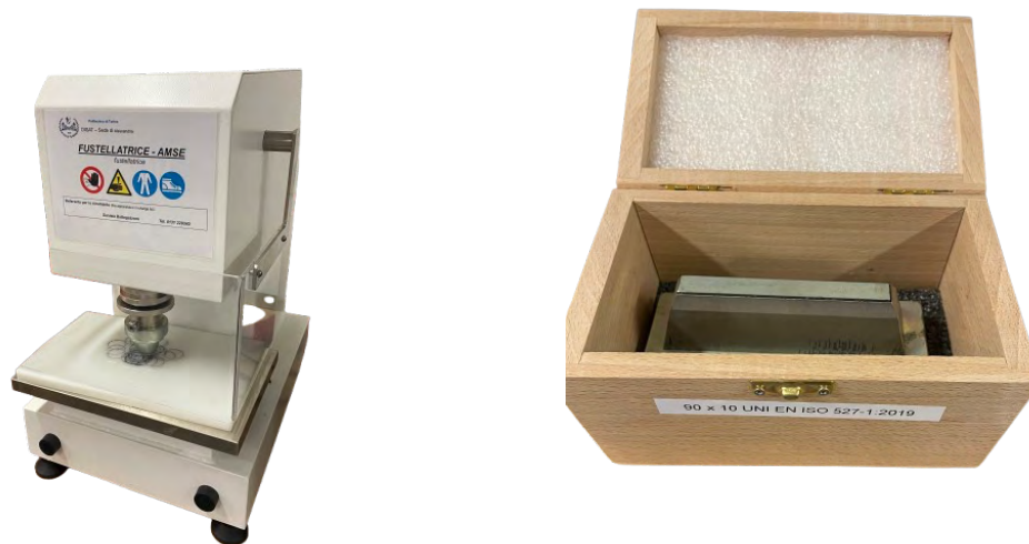
Fig. 13: the die cutter on the left and the die used to cut the samples into shape
