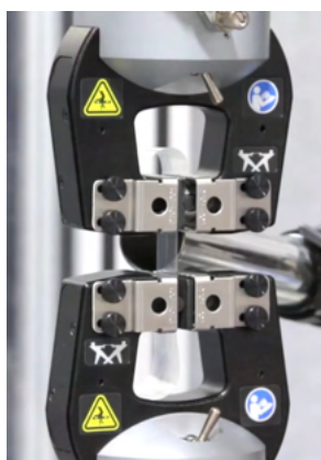
Fig. 15: Tensile test of a film following ASTM D882 standard [22]
