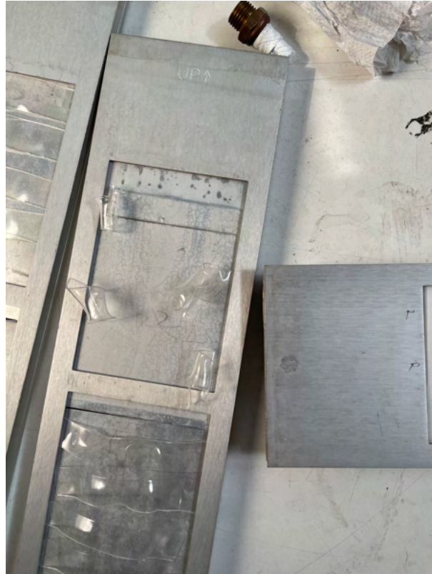
Fig. 25: PMMA/PLA 50/50 film coiling after going through QUV for 96 hours at 60 °C
