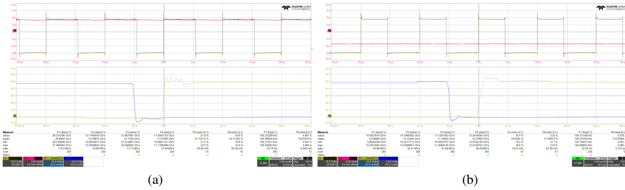
Figure 8.13: Switching node voltage measured on phase U at 48 V DC with 5 A (a) and -5 A (b) load current.
