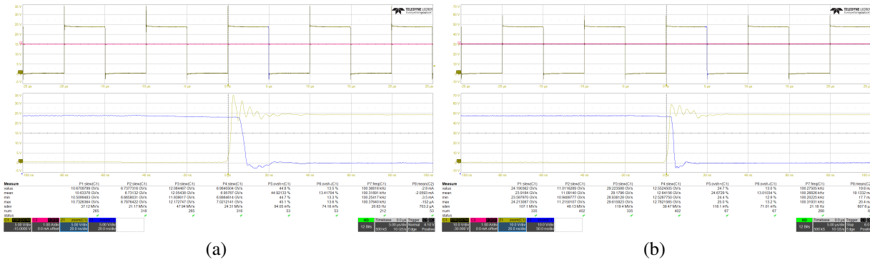
Figure 8.10: Switching node voltage measured on phase U at 24 V DC (a) and 48 V DC (b), with 0 A load current.
