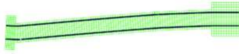
Figure 25: Beam's deformed shape right after bar fracture [5]
