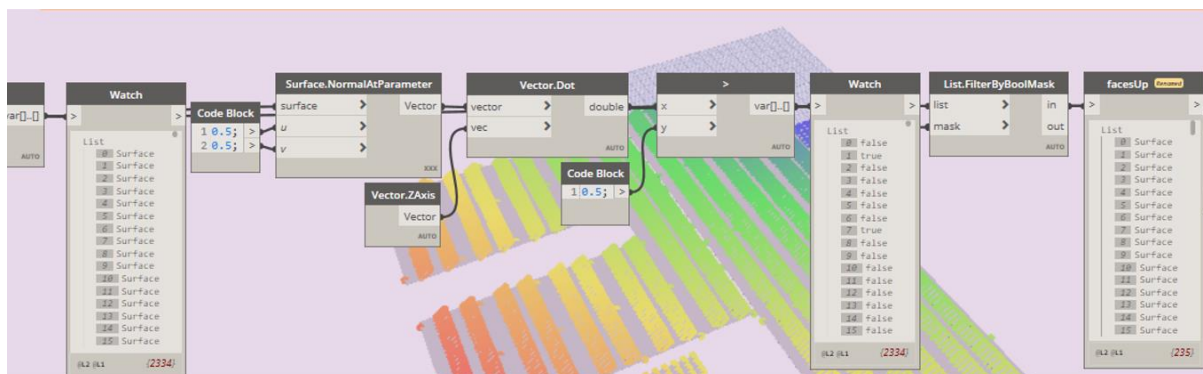
Figure 32 Dynamo algorithm executing vector dot product calculations to evaluate surface normals against the Z-axis, filtering out unsuitable faces into a refined group of valid host surfaces (facesUp).
