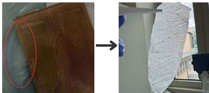
Figure 4.3. Immediate structural integrity loss of CA10_GVL membranes when immersed in the water bath due to instantaneous and violent liquid-liquid de-mixing rate.
