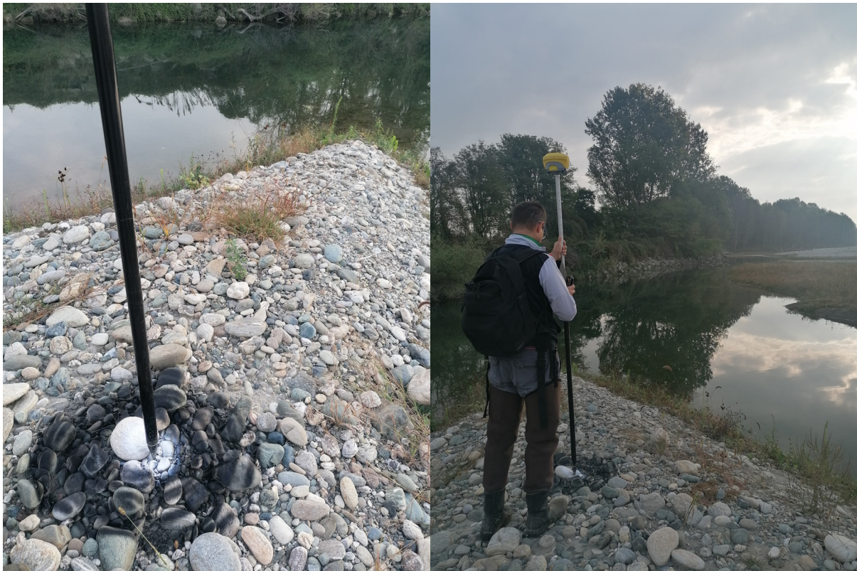
Fig.3 Ground Control Points realization during field survey using GNSS antenna and colored washable spray.
