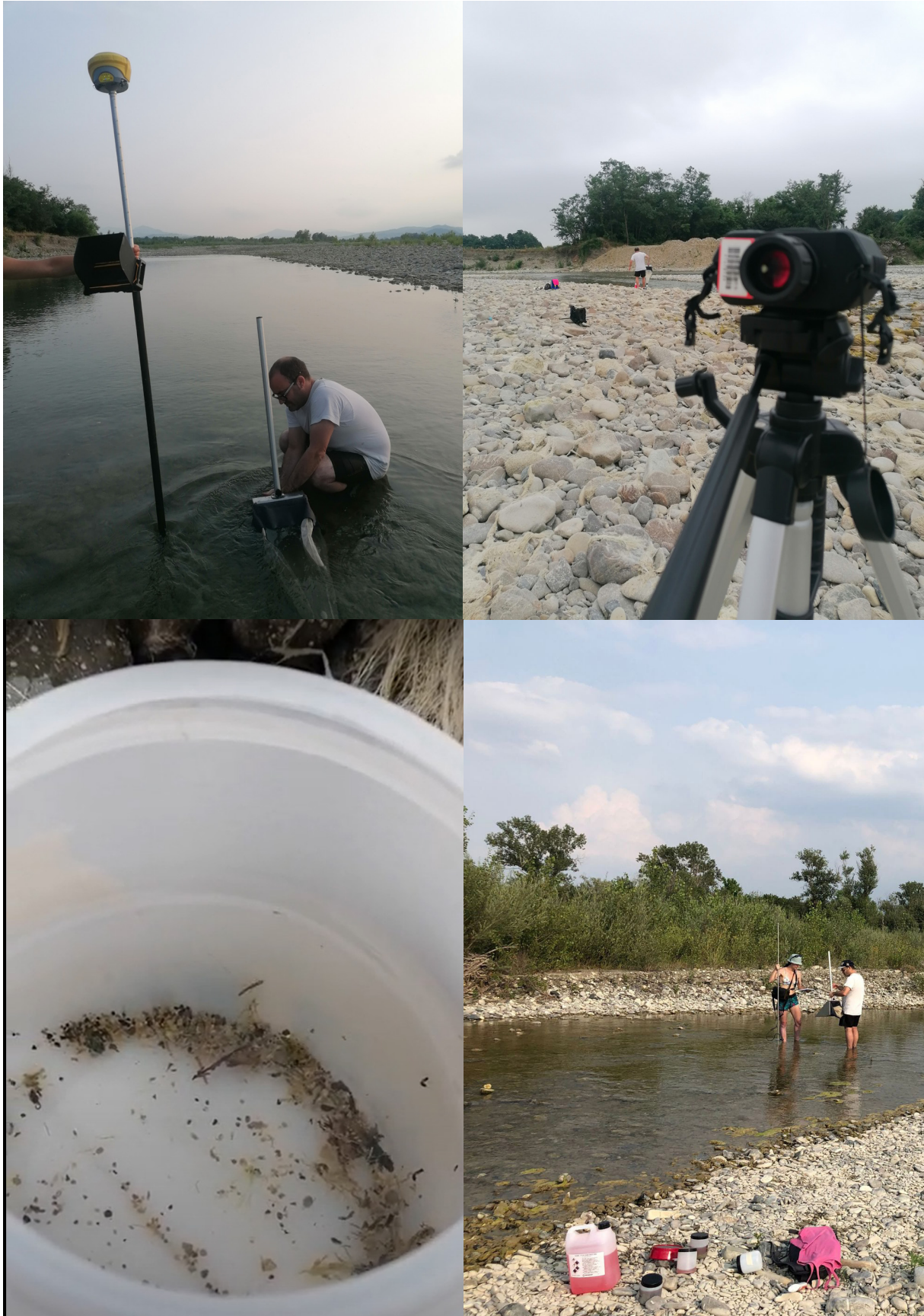
Fig.6 Up-left: Biological sampling with surber net and GNSS antenna. Up-right: rangefinder used for positioning when GNSS available not available. Down-left: Detail of a biological sample. Down-right: local depth and flow velocity description using current meter and paper notes. Also the alcohol and plastic jars for samples conservation and transport are visible.
