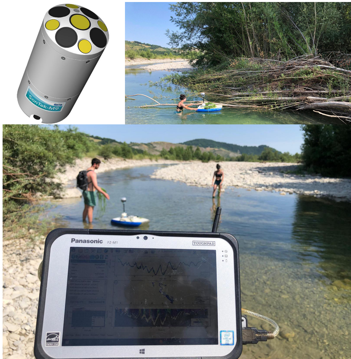
Fig.5 Up-left: River Surveyor M9 Acoustic Doppler sensor. Up-right: Bouyant platform containing the ADCP sensor and the GNSS antenna in use during field surveys. Down: River Surveyor Live software in use during field surveys.
