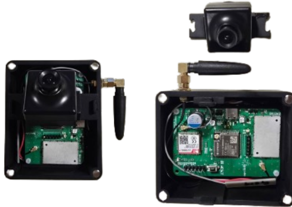
Figure 6.1. Fully assembled IxemCam wireless multimedia sensor node. The figure shows the final integrated hardware enclosed in a compact field-ready housing, including the ESP32-S3 control board, on-board SX1262 LoRa transceiver, cellular modem, camera module, and antenna interfaces. The assembled prototype demonstrates the feasibility of the proposed dual-radio architecture as a complete and deployable system rather than a laboratory-only design.
