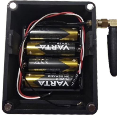
Figure 3.6. Battery enclosure used for field deployment, housing four AA alkaline LR6 cells arranged in a 2S2P configuration. The enclosure provides mechanical protection, strain relief for wiring, and a compact form factor suitable for outdoor operation.
