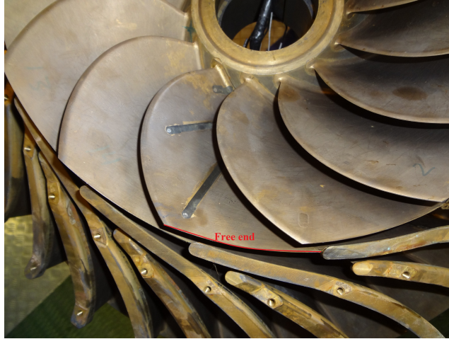
Figure 7.3: Francis-99 runner with free end trailing edge joined to band (marked in red color) [56]
