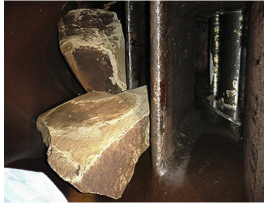
(b) Stones blocked in the spiral casing at the entrance of the stay vanes [31]
