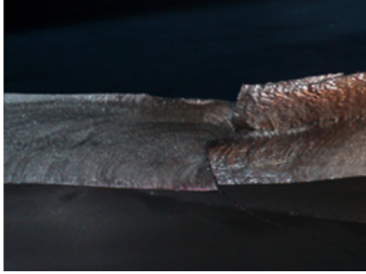
Figure 4.2: Fatigue damage on the runner with the bench marks [29]
