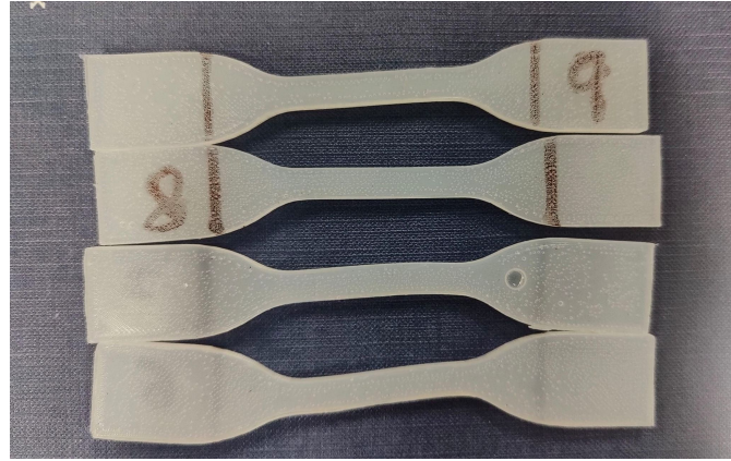
Figure 3.3: Some of the samples. It is slightly visible that the surface of the samples close to the top part of the mold shows some small air bubble. One of the samples even shows a bubble of important size that in this case, observing the curve obtained and the behavior during the loading, it's possible to assume it did not affected the results of the test.
