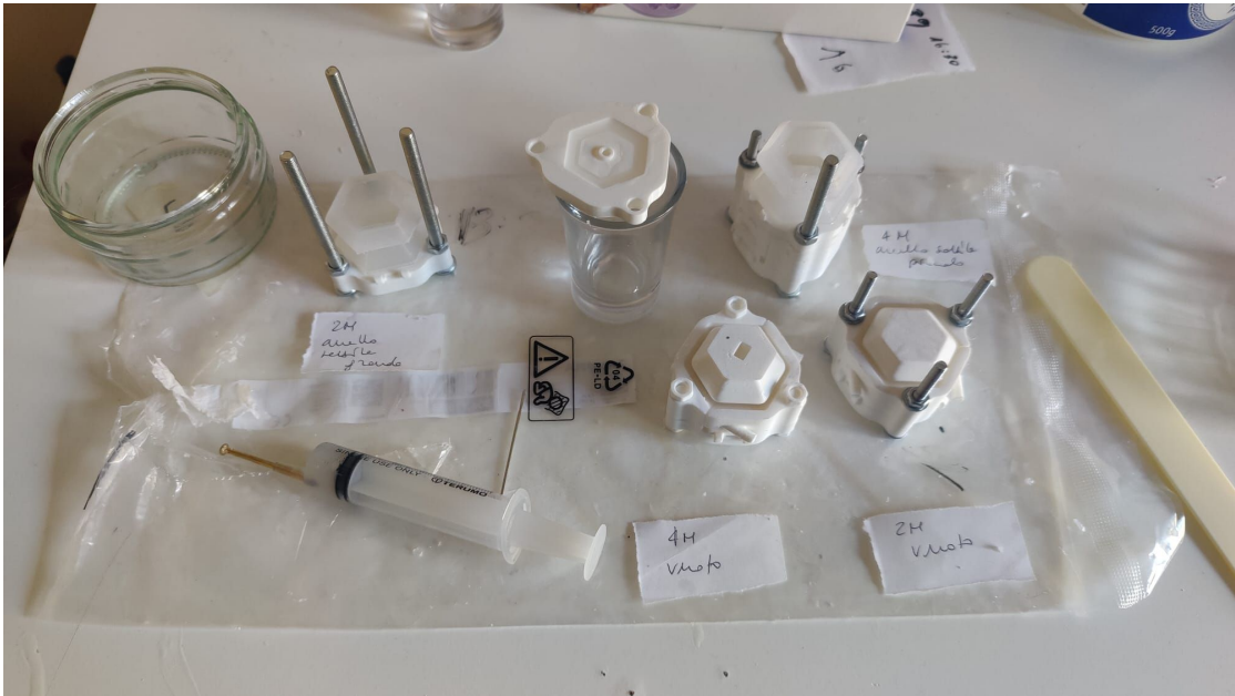
Figure 4.11: Working table during the fabrication campaign, showing samples at various stages of the production process and the auxiliary tools used.
