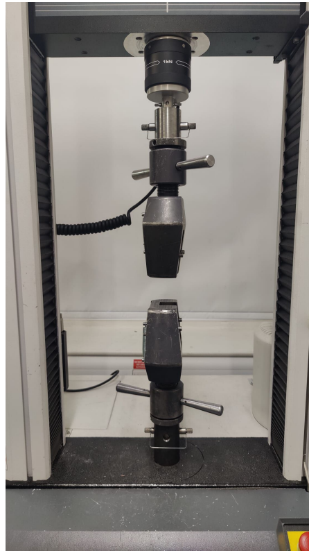
Figure 3.6: Experimental setup, detail of the 1kN fixture.
