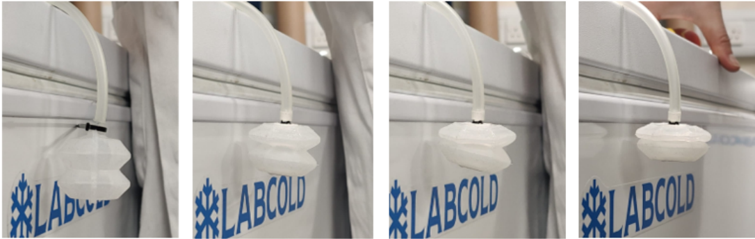
Figure 4.13: Frames from the dynamic behavior of the 2 units actuator during compression.
