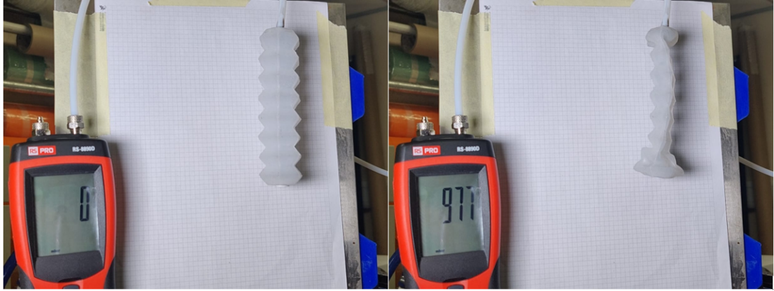
Figure 4.15: Initial and final frames from the 8-unit specimen under compression. Note that the deformed geometry of the “compressed” specimen deviates from the predicted shape, most likely due to the influence of self-weight.
