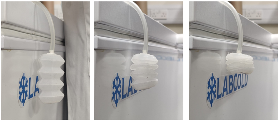
Figure 4.14: Frames from the dynamic behavior of the 4 units actuator during compression.
