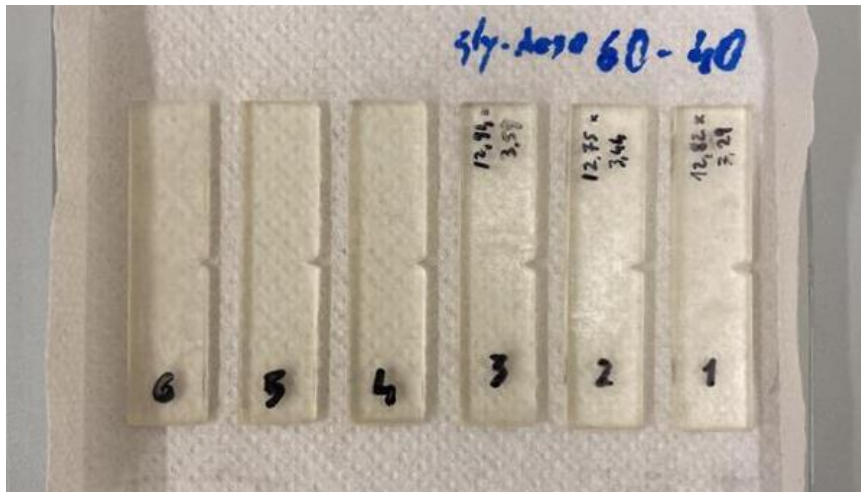
FIGURE 19 - 3D PRINTED NOTCHED SAMPLES (GLY/AESO:60-40 FORMULATION) USED IN THE IZOD IMPACT TESTS
