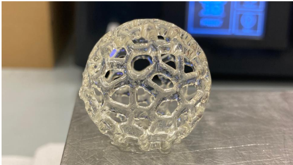
FIGURE 27 - HOLLOW SPHERE WITH VORONOI PATTERN (350 LAYERS - GLY/AESO:80-20)
