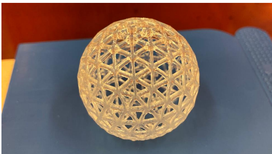
FIGURE 31 - HOLLOW SPHERE WITH GEODESIC PATTERN (350 LAYERS - GLY/AESO:70-30)
