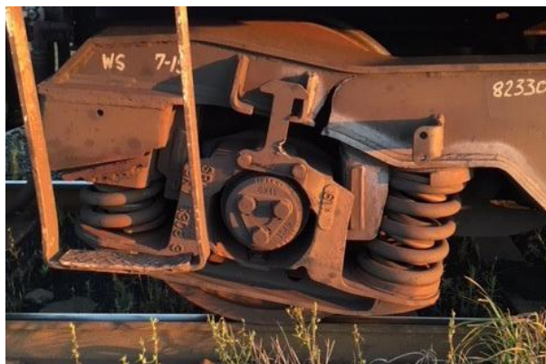
Figure 1Bogie fatigue cracking undetected during preventative maintenance (Source : ASTB Gov)
