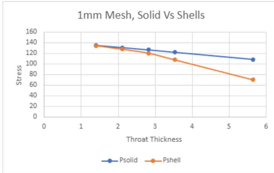
Figure 19 ; Solid to shells for 1mm mesh size , (Source - Author)
