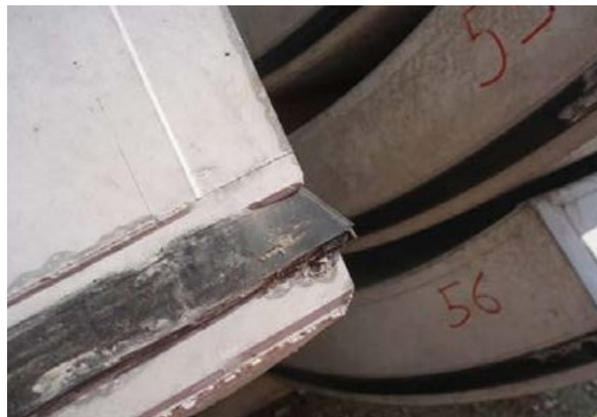
Figure 15 Corner Gasket Damage (SIG WG2, 2019)
