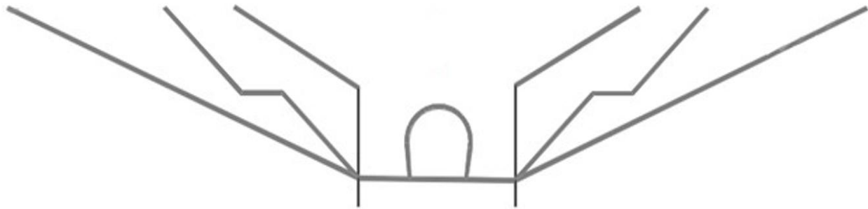
Figure 28 Figure that shows the slope, slope with berm, and slope coupled with vertically retained slope
