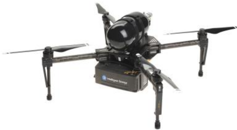
Figure 15: Intelligent Energy's fuel cell prototype system mounted in UAV
