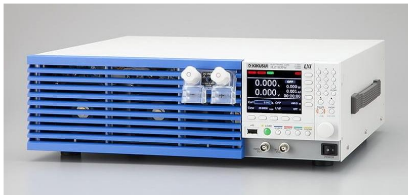
Figure 21: Kikusui PLZ1205W electronic load [57]
