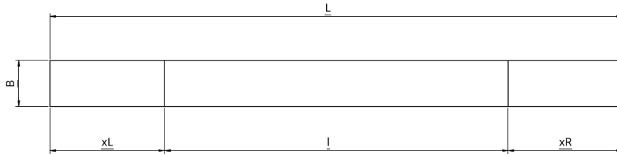
Figure 3.6: Geometry of the \pm 60^\circ tensile specimen.
