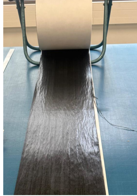
(d) Prepreg material roll used for specimen manufacturing.
