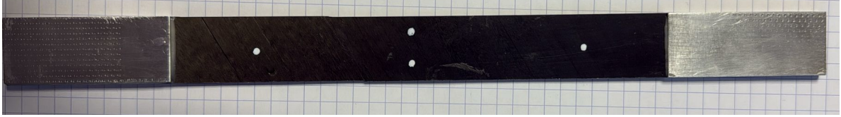
(b) Real specimen with the optical tracking reference dots.
