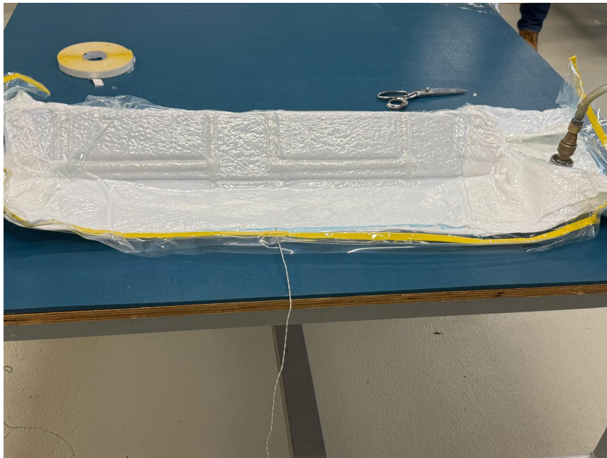
Figure A.2: Vacuum bagging configuration prepared before the curing cycle.
