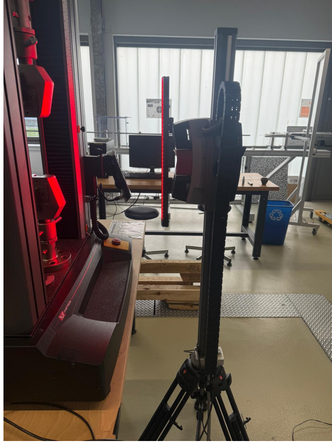
Figure 3.8: Optical acquisition system used to track the displacement of the reference dots during the tensile test.
