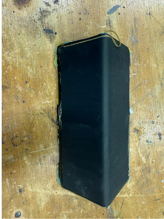
Figure A.5: Demoulded L-shaped composite specimen after the curing process.
