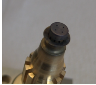
Figure 2.11: Deflector and a cooled pintle tip [20]
