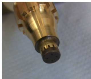
Figure 2.9: Active cooling system incorporated for pintle tip[20]
