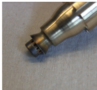
Figure 2.10: Deflector for displacement of the impingement point[20]
