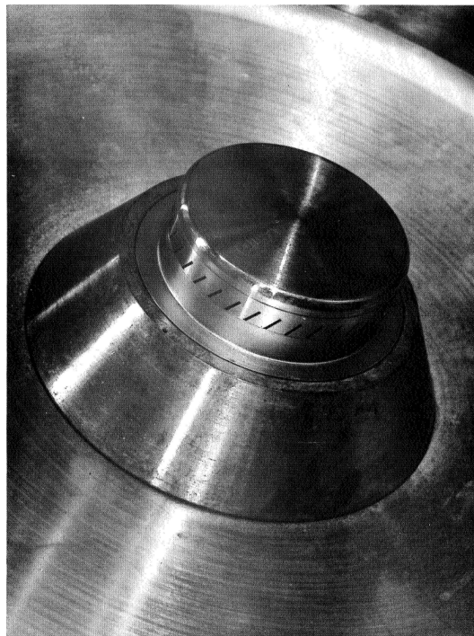
Figure 2.12: Canted slot configuration[18]
