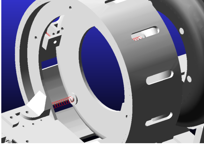
Figure 6.7: Rear detail of the female docking interface. Notice the position of springs (two longitudinal and one perpendicular are visible) and the absence of screws, nuts and washers in the visualization.
