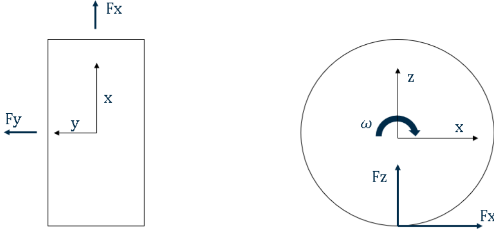
Figure 2.6: Local wheel reference frame \mathcal{W}_i : top view (left) and side view (right) showing internal axes, angular velocity, and acting forces.
