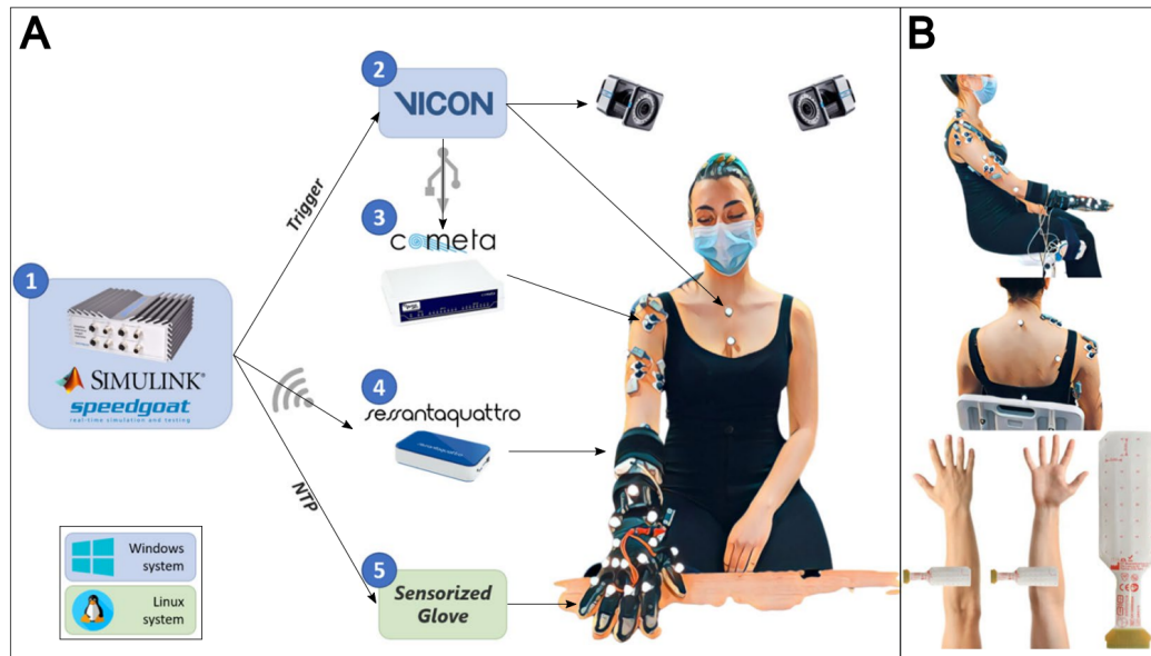
Figure 5.1: Experimental setup. (A) 1) Real Time target machine Speedgoat running the Simulink model. 2) Vicon motion capture system. 3) Cometa system bipolar EMG. 4) Sessantaquattro high-density EMG. 5) Sensorized glove from Bielefeld University. (B) Placement of the acquisition sensors: 23 reflective markers for the Vicon system, 10 bipolar EMG electrodes, 2 grids for HD-sEMG acquisition, and sensorized glove[7].
