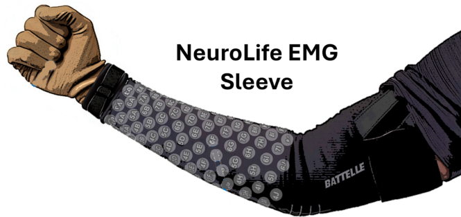
Figure 3.2: High-density EMG sleeve interface. The NeuroLife® sleeve features a dense grid of up to 150 embedded electrodes covering the entire forearm circumference. This configuration enables the high-resolution capture of spatiotemporal muscle activation patterns from both superficial and deep muscle groups, providing a rich dataset for decoding complex hand gestures and continuous joint kinematics compared to traditional sparse electrode setups. [65].
