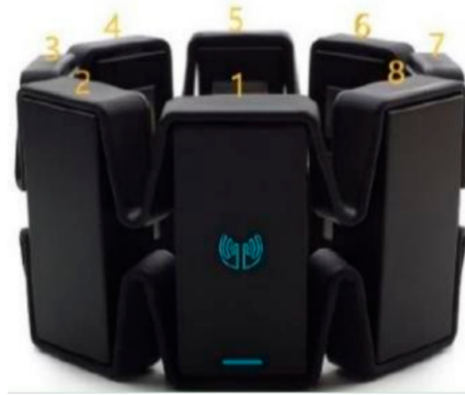
Figure 3.1: Low-density EMG armband for gesture recognition. The Myo armband (Thalmic Labs) features a sparse circumferential array of 8 dry bipolar sEMG sensors. This configuration is representative of commercial low-density interfaces, providing discrete muscle activity signals for classifying hand gestures with low computational overhead and setup time [62].
