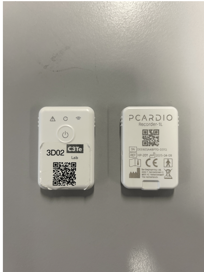
Figure 3.1: P-Cardio recorders (50x35x9mm, 20gr).
