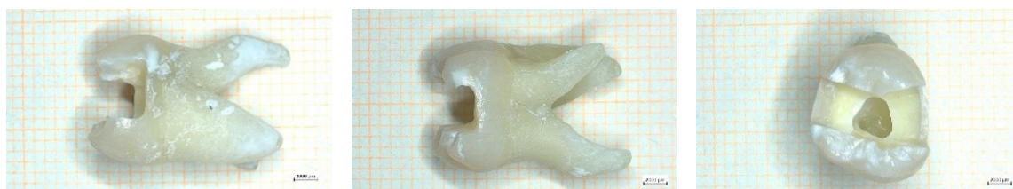
(a) 4 mm deep dental cavity preparation (b) 2 mm deep dental cavity preparation (c) Occlusal view of both cavity preparations performed on a tooth specimen without the application of dental adhesive pre-treatment
