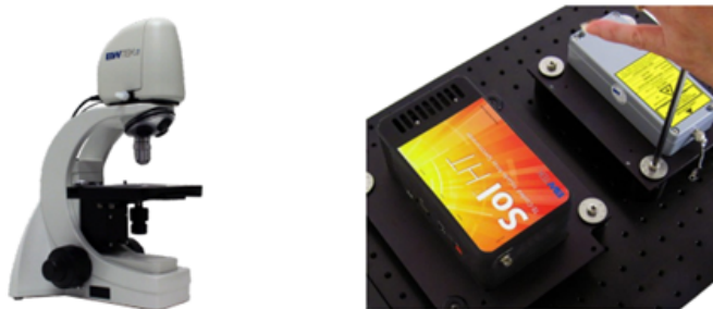
Figure 2.7: Portable modular Raman spectrometer (BWTEK) equipped with a BTC284N detector and a 1064 nm laser source, coupled with the BAC151 compact microscope used for sample observation and laser focusing.
