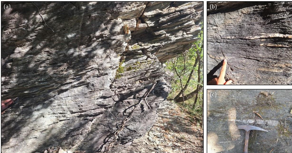
Figure 7.7 - Geomechanical survey photos; (a) schistosity, (b) and (c) quartz veins.
