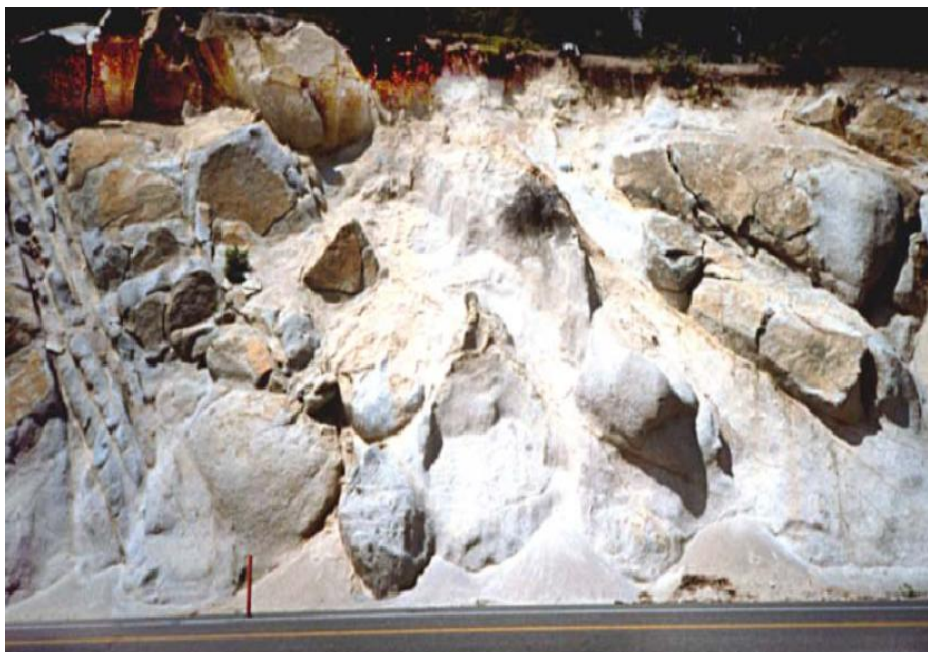
Figure 2.3 Example of a mélange deposit characterized by a chaotic block-in-matrix structure (after Medley, 2001).
