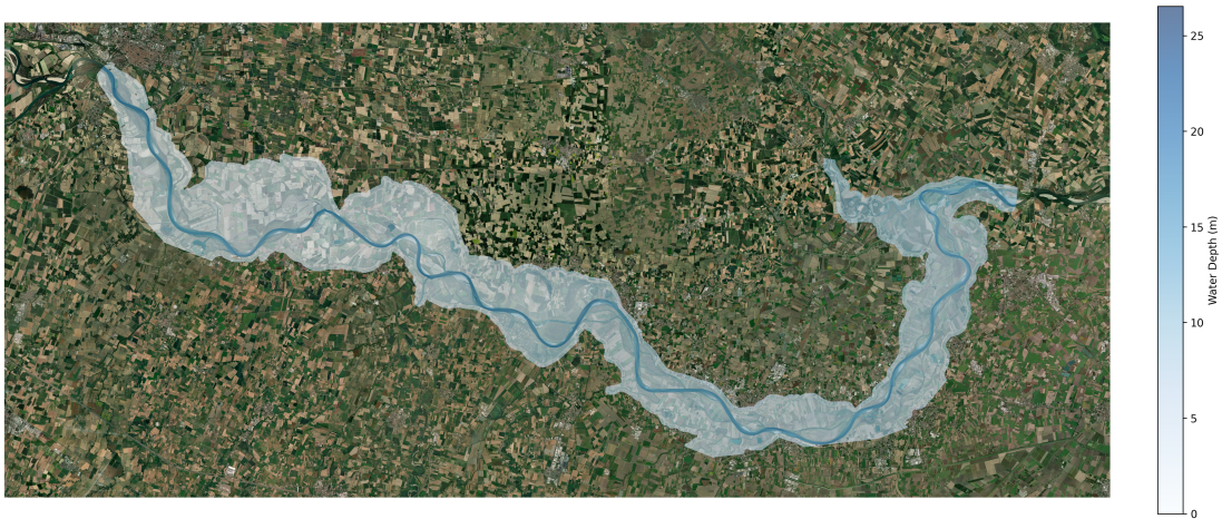
Figure 41: Global Inundation Map: Modeled Po River reach from the HEC-RAS Q = 8200 \text{ m}^3/\text{s} flood event simulation results, overlaid on satellite imagery.
