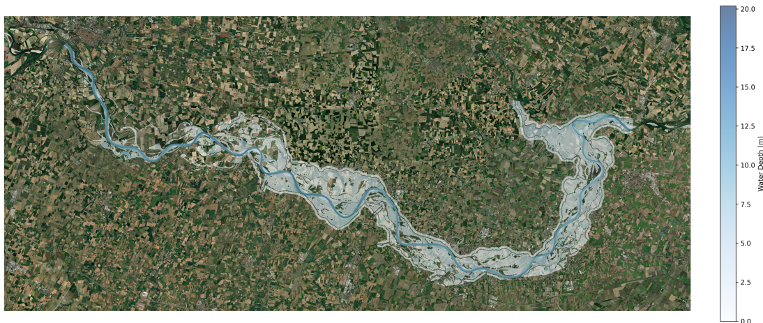
Figure 40: Global Inundation Map: Modeled Po River reach from the HEC-RAS Q = 8200 \text{ m}^3/s flood event simulation results, overlaid on satellite imagery.
