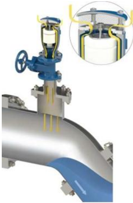
Figure 46: scheme of air valve that lets air in due to pipe emptying (source: Vesipa R. Civil and industrial hydraulic systems – Lectures material, 2025)
