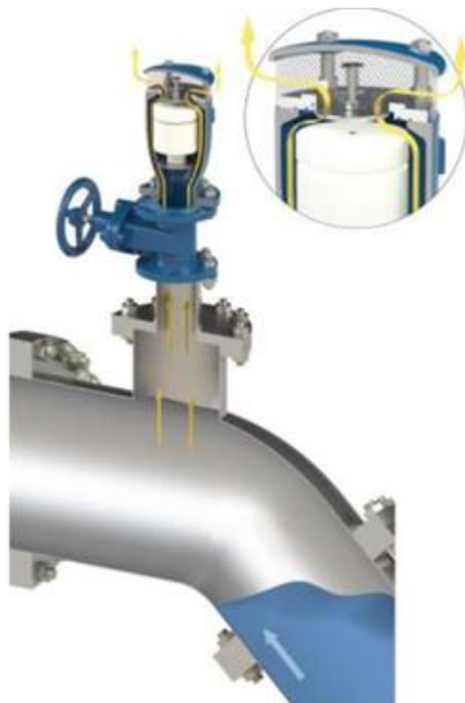
Figure 47: scheme of air valve that lets air out due to pipe filling (source: Vesipa R. Civil and industrial hydraulic systems – Lectures material, 2025)
