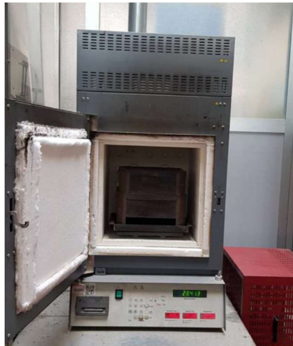
Figure 28 Ignition furnace used for the determination of binder content
