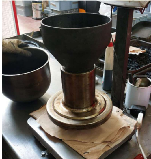
Figure 25 Placement of asphalt mixture into the mould
