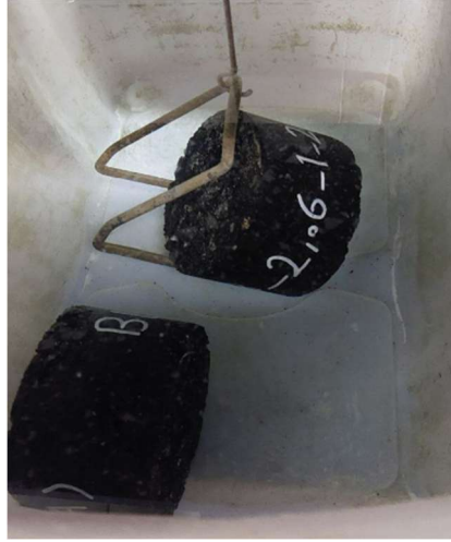
Figure 37 Asphalt specimen suspended in water for determination of submerged mass [28].
