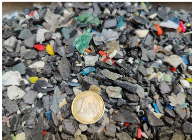
Figure 17 Waste plastics MEGPO used in the experimental mixtures
