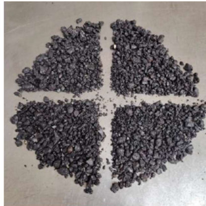
Figure 26 Quartering of the loose asphalt [25].
