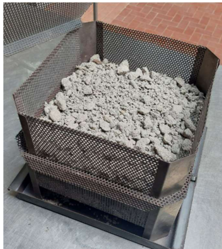
Figure 30 Aggregates remaining after binder combustion during the ignition test
