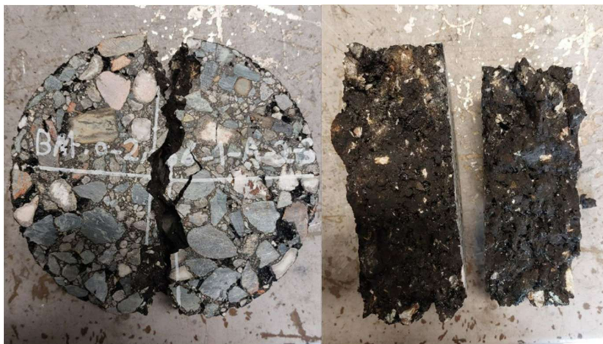
Figure 44 Failure pattern after the ITS test: (L) diametral crack; (R) fracture surfaces along the loading diameter.
