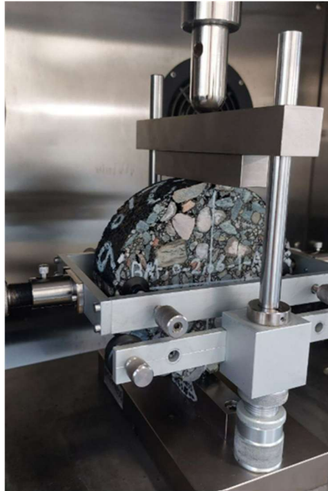
Figure 42 Experimental setup for the ITS test [30]
