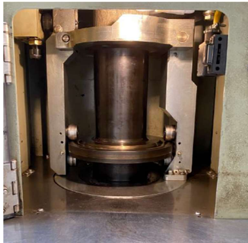
Figure 31 Superpave Gyratory Compactor used for specimen preparation
