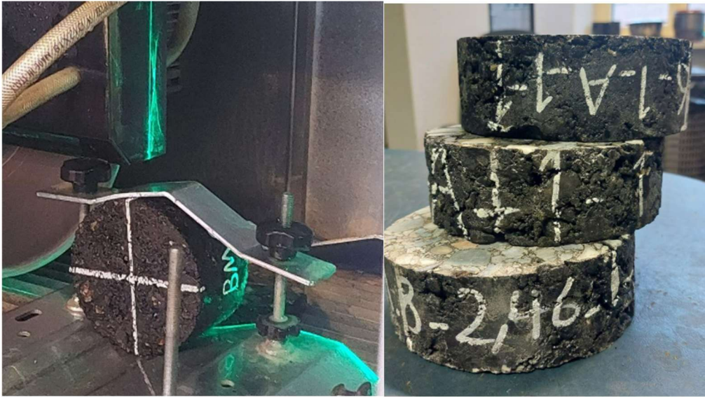
Figure 36 Cutting of gyratory-compacted specimens and cut specimens
