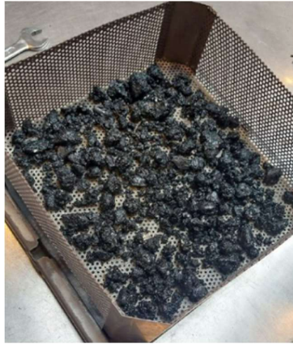
Figure 29 Metallic basket containing the loose asphalt mixture before the ignition test
