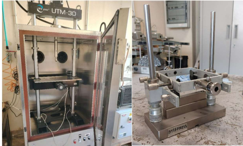
Figure 39 Universal Testing Machine (UTM) used for the mechanical testing of asphalt specimens.
