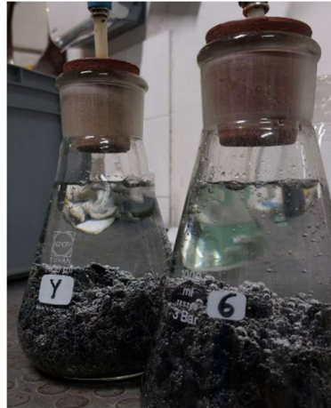
Figure 27 Pycnometer apparatus used for the determination of the maximum theoretical density
