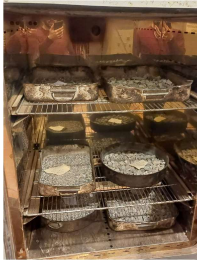
Figure 22 Heating of aggregates prior to mixing
