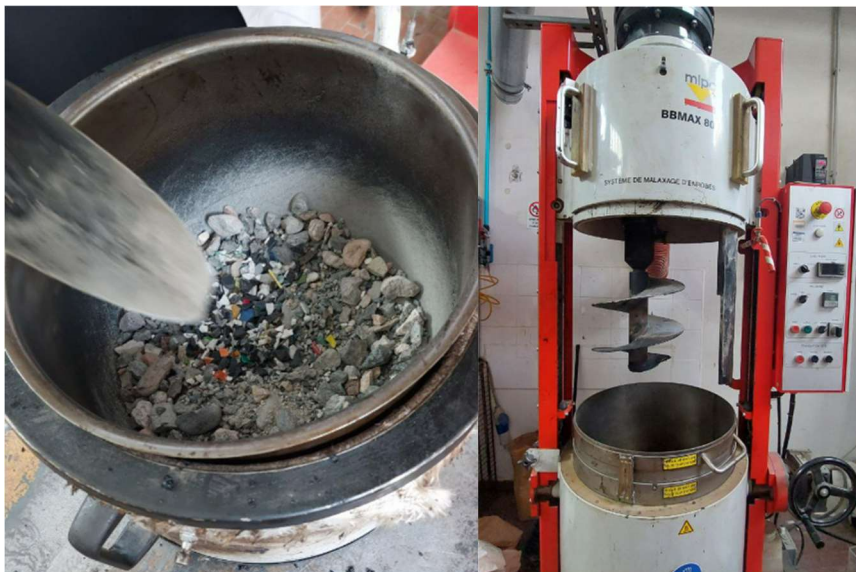
Figure 24 Mixing procedure of the asphalt mixture in the laboratory
