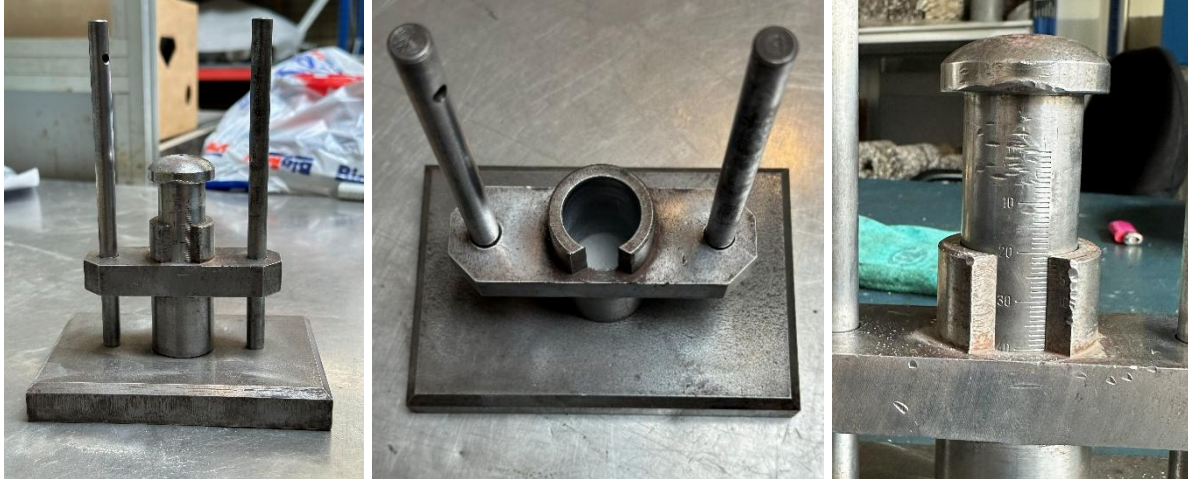
Figure 5 – Rigden void test apparatus
