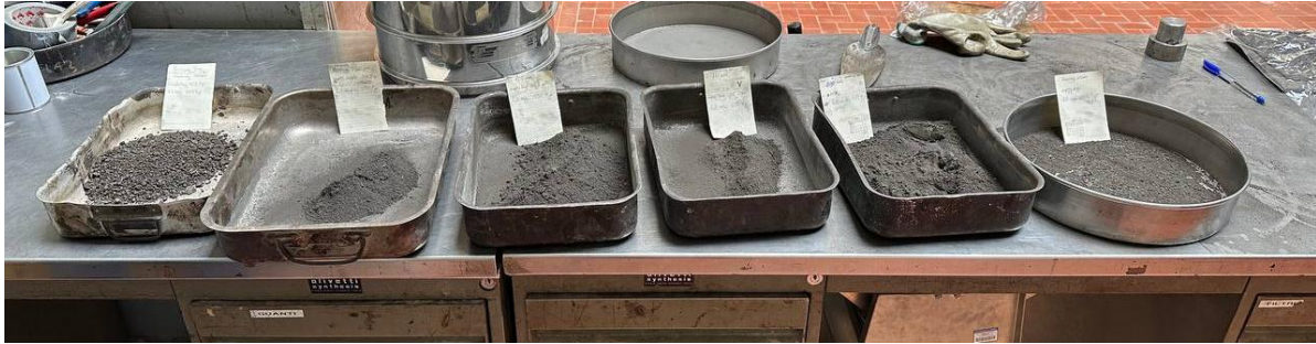
Figure 2 – Different particle size of fillers derived from sieving method
