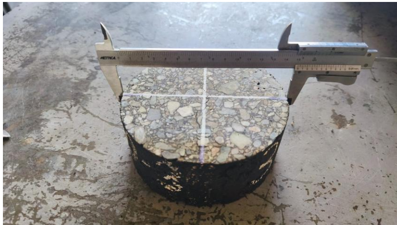
Figure 44. Detail of the height measurement of a cylindrical specimen
