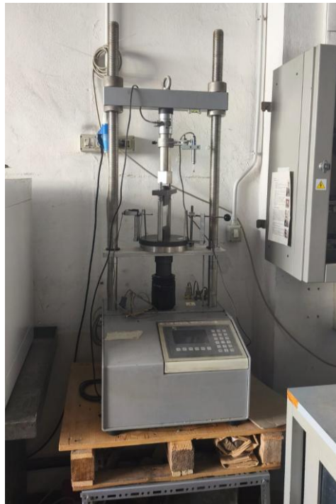
Figure 57. ITS testing system
