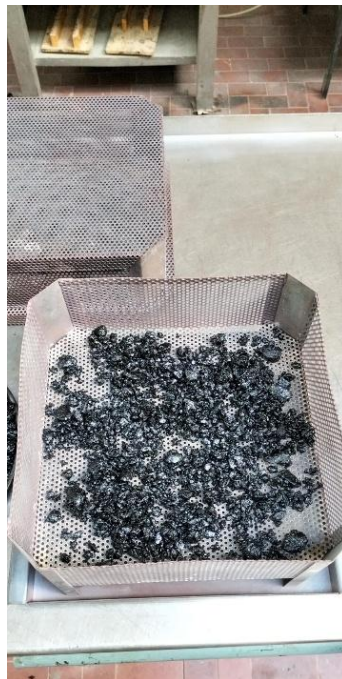
Figure 33. Mass of the basket and the sample before ignition, expressed in g, W_{t+s} .
