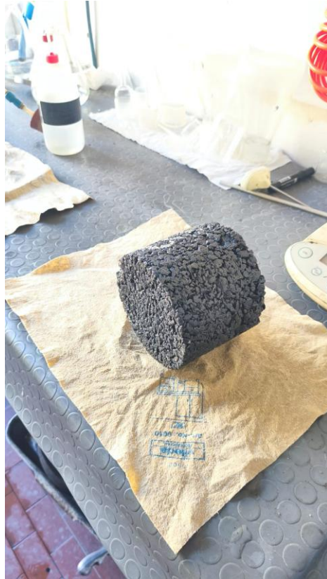
Figure 49. Drying of the specimen external surface with a dry chamois cloth
