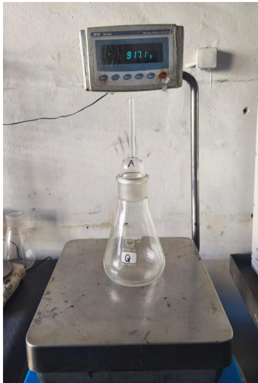
Figure 24. Weighing of the pycnometer, with known calibrated volume, and its cap, m_1 .
