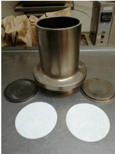
Figure 38. Mould with appropriate metal inserts and filter paper sheets
