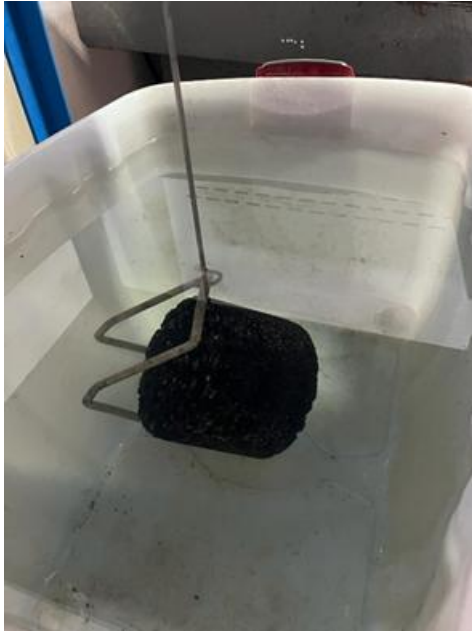
Figure 48. Recording of the specimen mass in water, known as m_2 .
