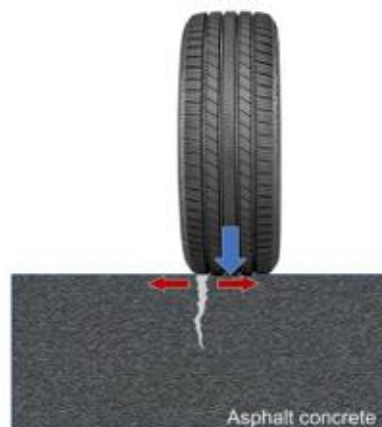
Figure 8. Top down cracking (source: Bessa et al., 2022)
