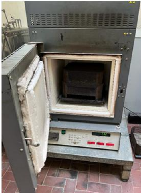
Figure 34. Introduction of the basket, with material, into the oven
