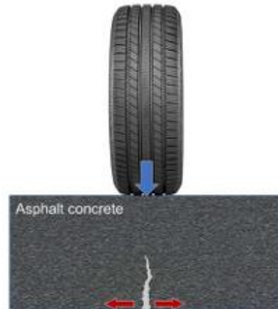
Figure 9. Bottom up cracking (source: Bessa et al., 2022)
