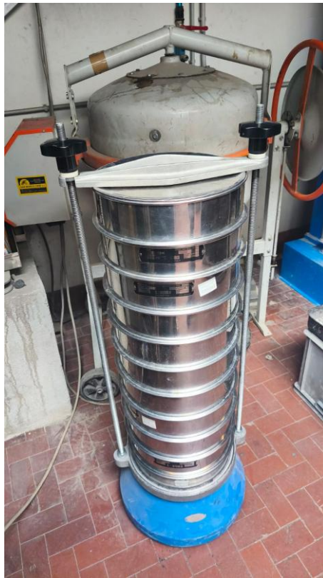
Figure 30. Sieve column mounted on a vibrating plate.
