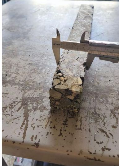
Figure 45. Detail of the geometric dimensions measurement of a prismatic specimen
