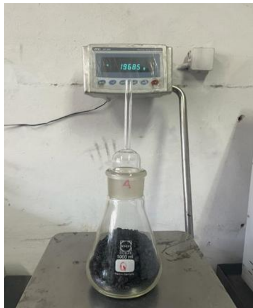
Figure 25. Weighing of the pycnometer, its cap and the dry material sample, m_2 .
