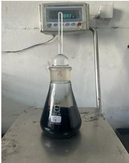
Figure 27. Weighing of the pycnometer, its cap, the sample and water filled to the meniscus, m_3 .
