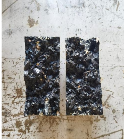
Figure 59. Detail of the fracture of a specimen after the ITS test.
