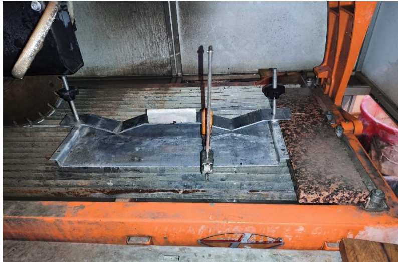
Figure 42. Detail of a self-made guide used to properly cut the material slabs.
