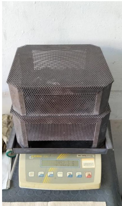
Figure 32. Perforated basket for containing the material and a collection tray for the residues
