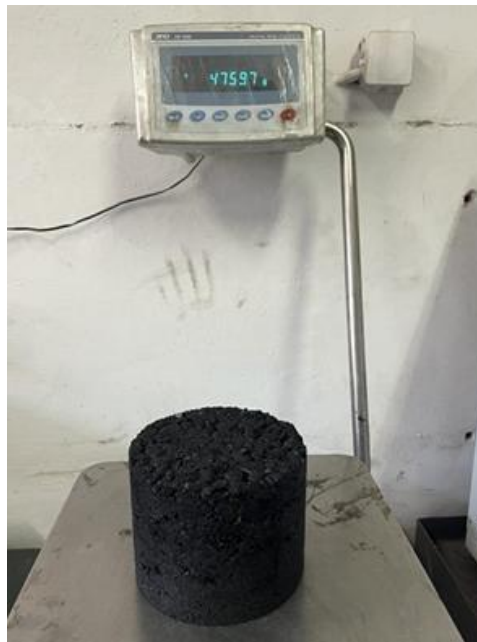
Figure 46. Recording of the dry specimen mass, referred to as m_1 .
