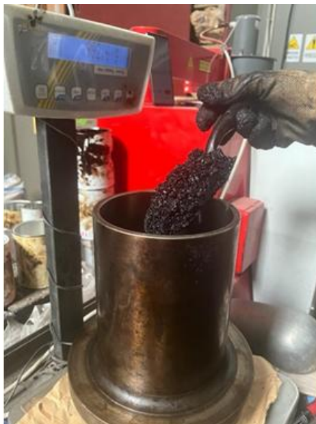
Figure 40. Insertion of the bituminous mixture inside the mould, positioning a filter paper sheet at the base
