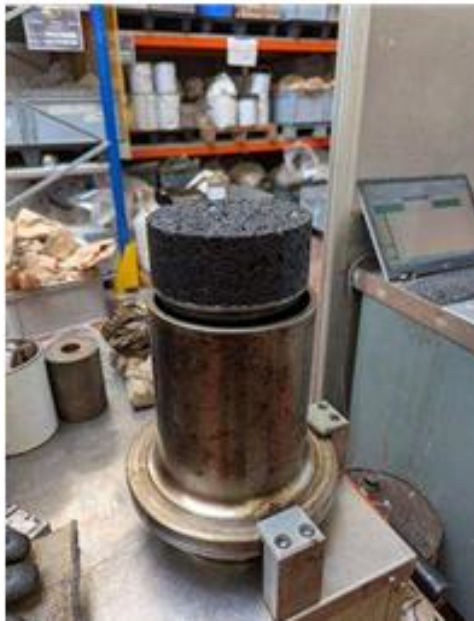
Figure 41. Removal of the freshly compacted specimen by extruding it from the mould using a hydraulic piston
