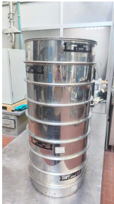
Figure 29. Sieve stack for performing the sieve analysis.
