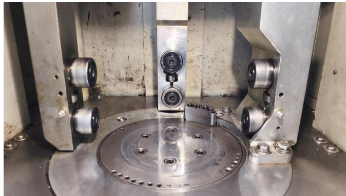
Figure 39. Positioning of the mould inside the appropriate housing of the gyratory shear press and fixing to the three clamps located inside the machine chamber
