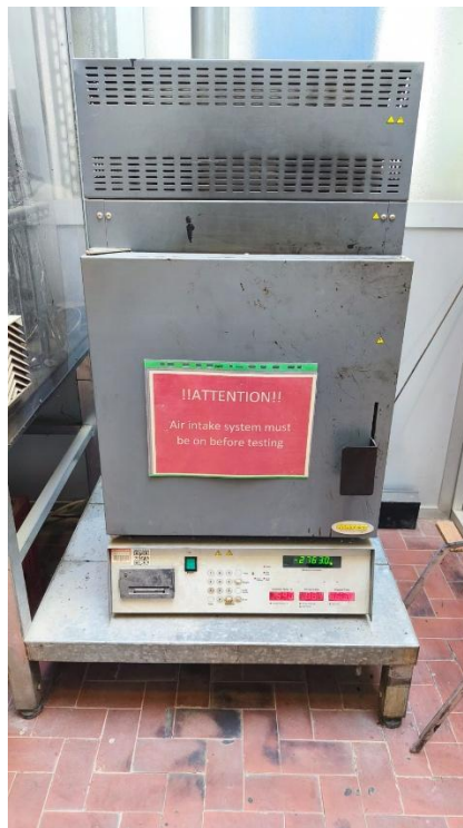
Figure 31. Oven capable of reaching the test temperature, 540 °C
