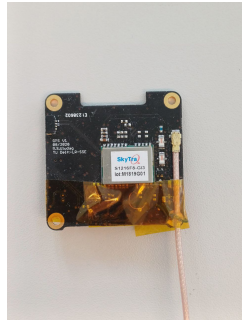
Figure 4.3: SkyTraq PX1122C Single Frequency GNSS Receiver installed on its board
