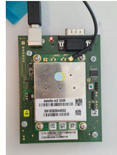
Figure 4.4: Septentrio AsteRx-m2 OEM Dual Frequency GNSS Receiver installed on its board
