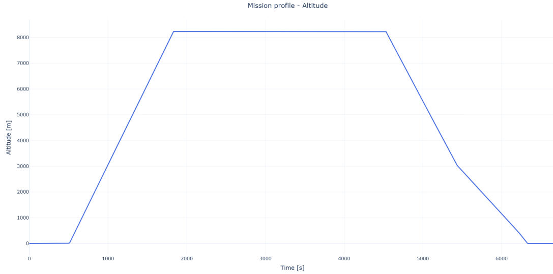
Figure 3.25: Altitude curve for the mission profile in table 3.2
