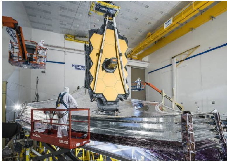
Figure 5.1: The sunshield of the James Webb Space Telescope (JWST), demonstrating a critical application of high-performance polymers in space structures. The membranes are composed of Kapton polyimide relied upon for its thermal stability but requiring specialized coatings for environmental protection.
