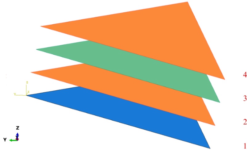
Figure 6.2: Layered configuration of the composite plate illustrating the arrangement of CFRP (blue), copper foil (orange), and RT/Duroid 5880 dielectric (green) layers
