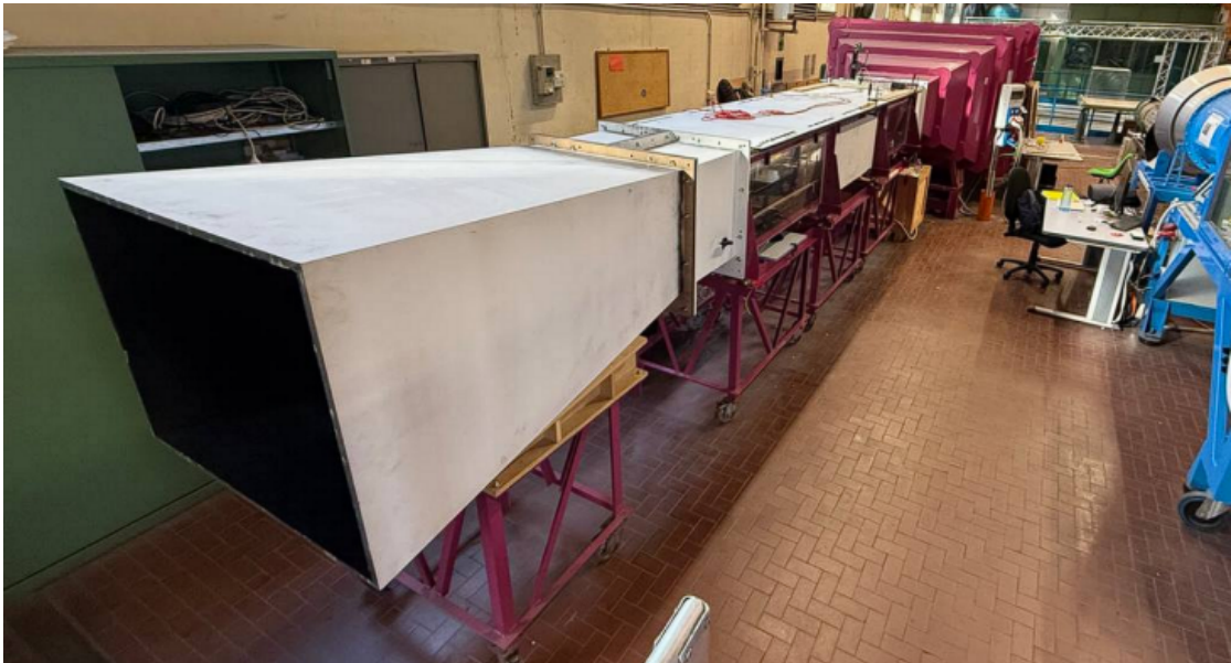
Figure 3.5: The Fuxia wind tunnel of Laboratory of Aeronautics M. Panetti of Politecnico of Torino.
