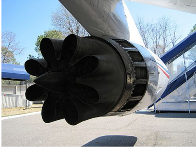
(a) Hush kit mixer on the turbojet General Electric CJ805
