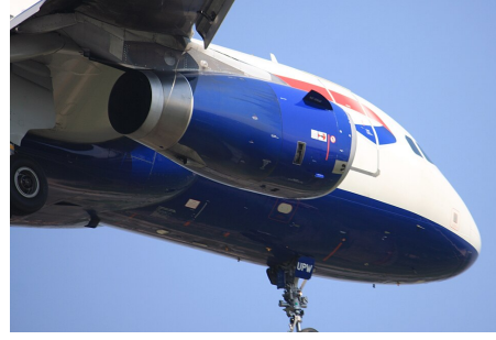
(b) The IAE V2500 on the A320 family, using a mixed exhaust
