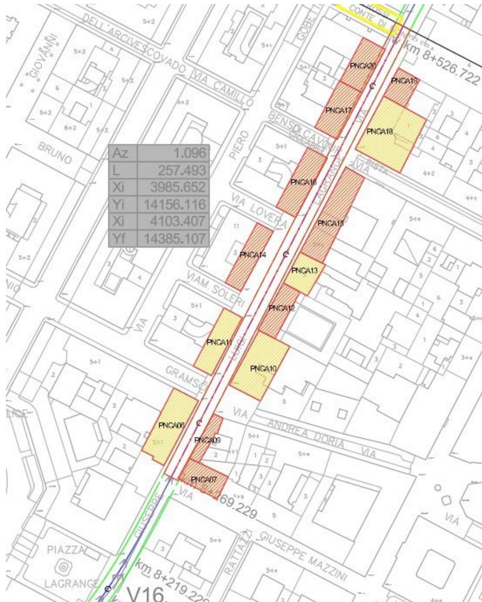
Figure 5.2. Planar view of analyzing section with underlined buildings for damage assessment
