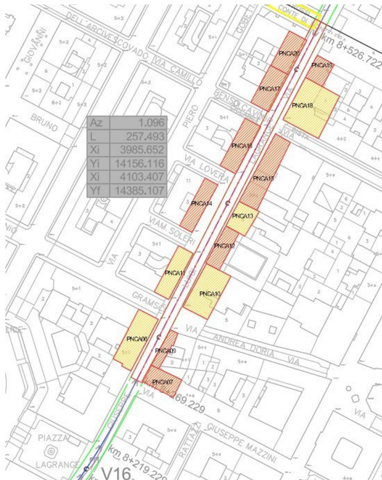
Figure 6.25. Planar view of analyzing section with underlined buildings for damage assessment
