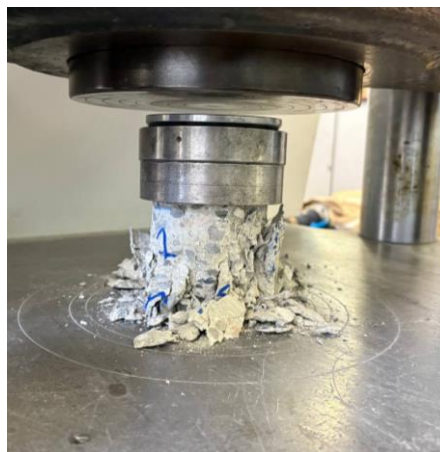
Figure 3-15: Specimen after failure under compressive load.
