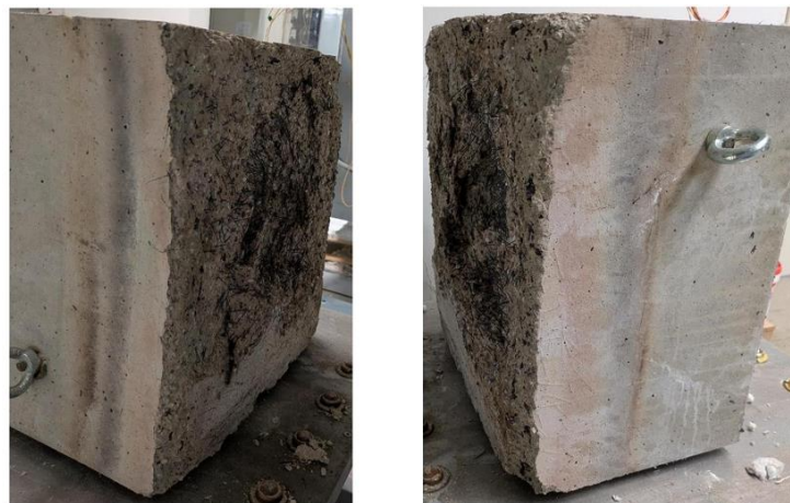
Figure 4-8: PP specimen after fire exposure.
