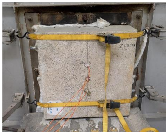
Figure 3-6: Specimen set-up in the furnace.
