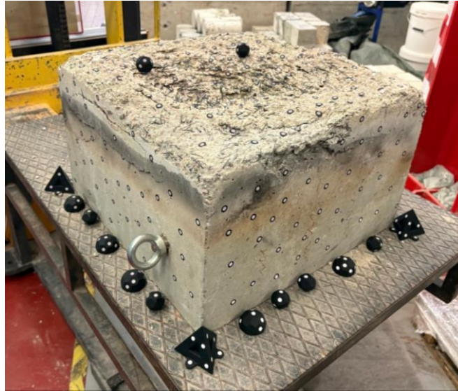
Figure 3-9: Example of marked specimen ready for scanning.
