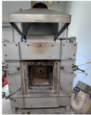
Figure 3-5: Furnace equipped with a single burner (J.F. Amonn s.r.l.).
