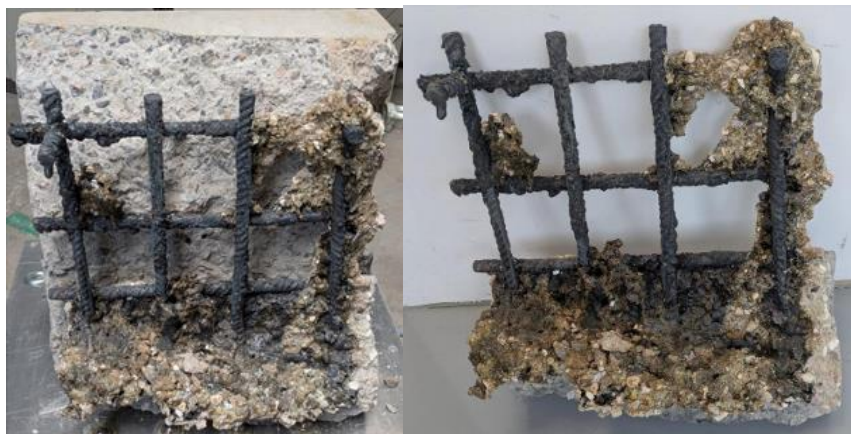
Figure 4-6: ARM specimen after fire exposure.
