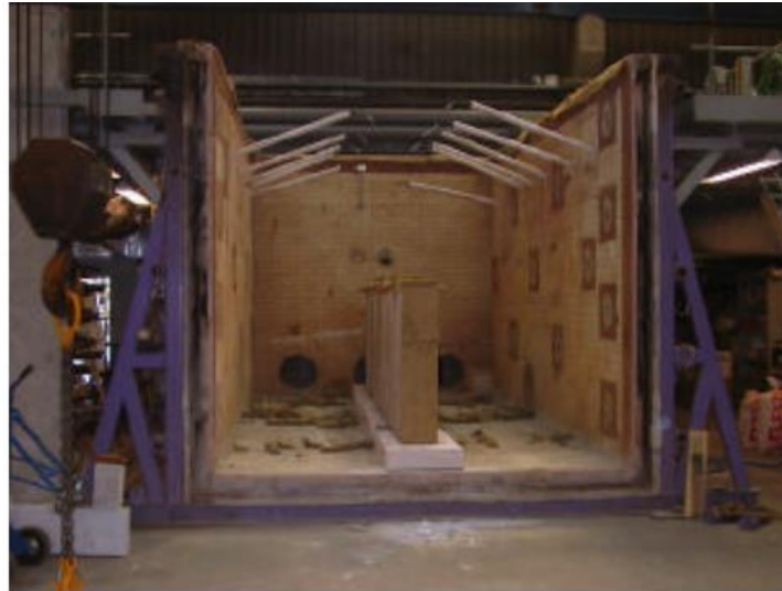
Figure 2-16[33]: Testing set-up for concrete wall elements.
