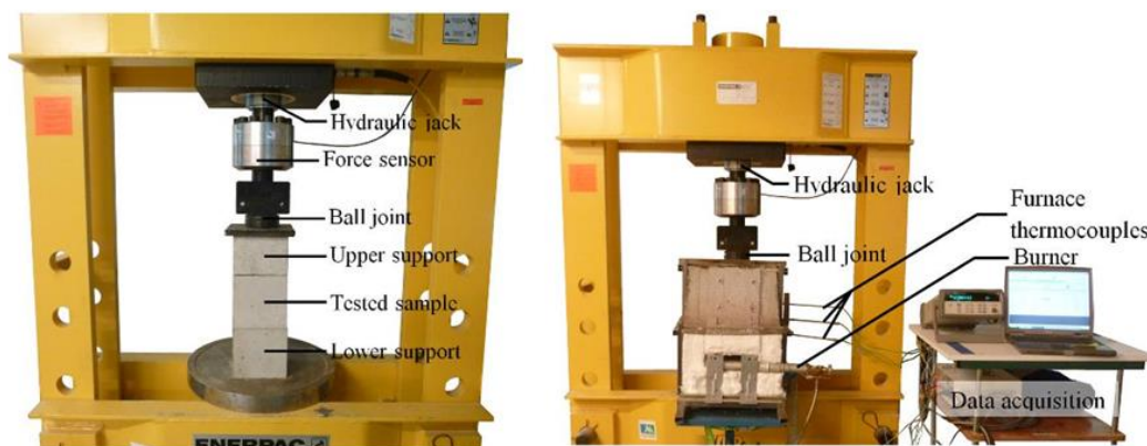
Figure 2-7[22]: Tested sample in the hydraulic press (left) and complete test setup (right).
