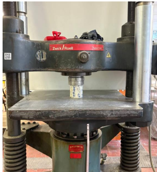
Figure 3-14: Compressive test set-up.
