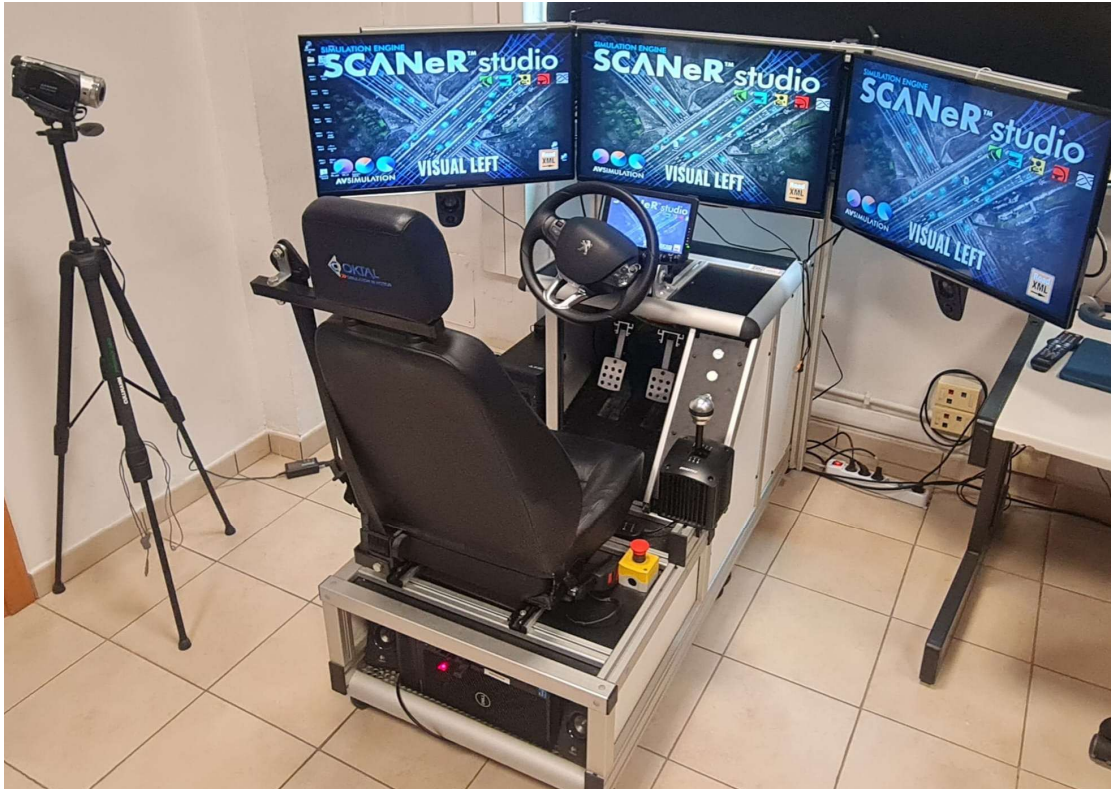
Figure 3.15 : Fixed-base driving simulator at RSDS Lab (Politecnico di Torino)
