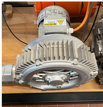
(a) Upstream blower
