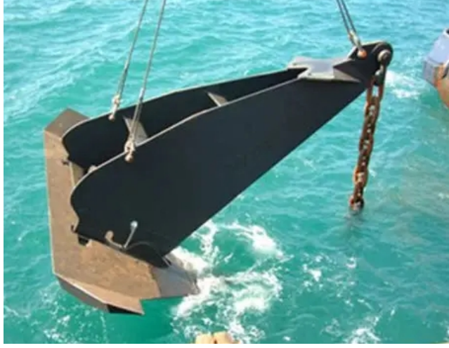
Figure 44: Example of a Drag Embedment Anchor.
