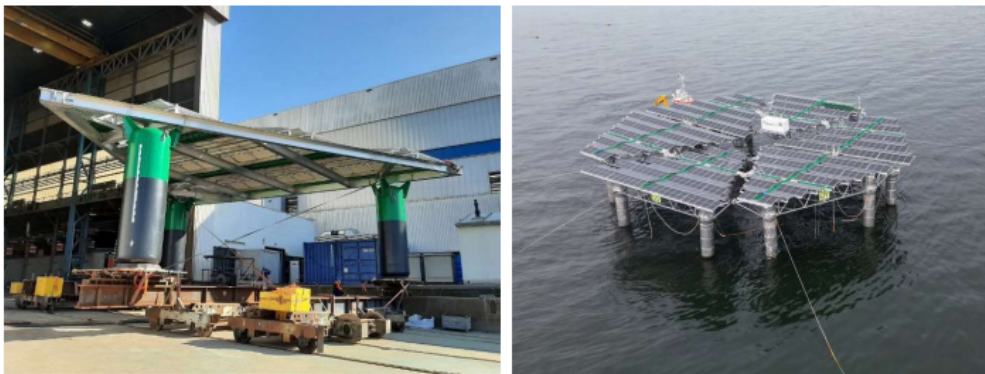
Figure 2.3: Examples of individual floater units and interconnected floating island configurations used in semi-submerged rigid FPV systems (source [7]).
