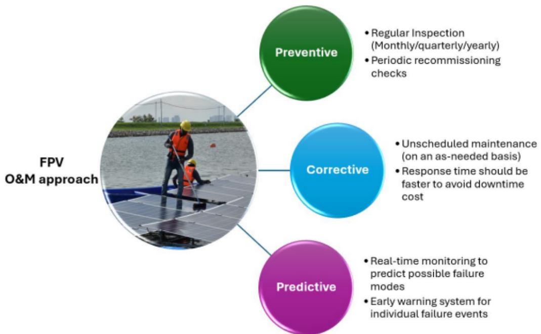
Figure 5.10: Illustration of O&M approach for FPV systems (source [75]).
