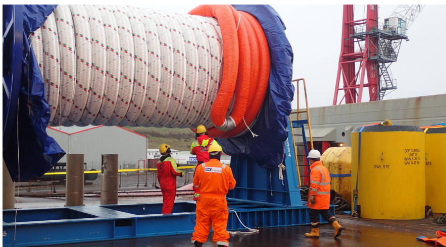
Figure 5.5: Example of synthetic ropes for offshore application (source [63]).
