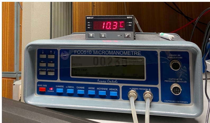
Figure 28: The micromanometer that provides the pressure, and the thermometer of the wind tunnel chamber
