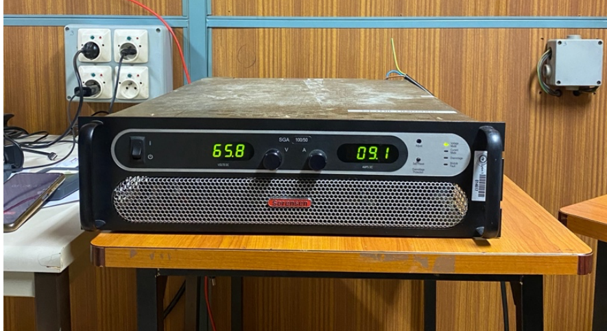
Figure 30: DC power supply (Sorensen SGA 100/50)
