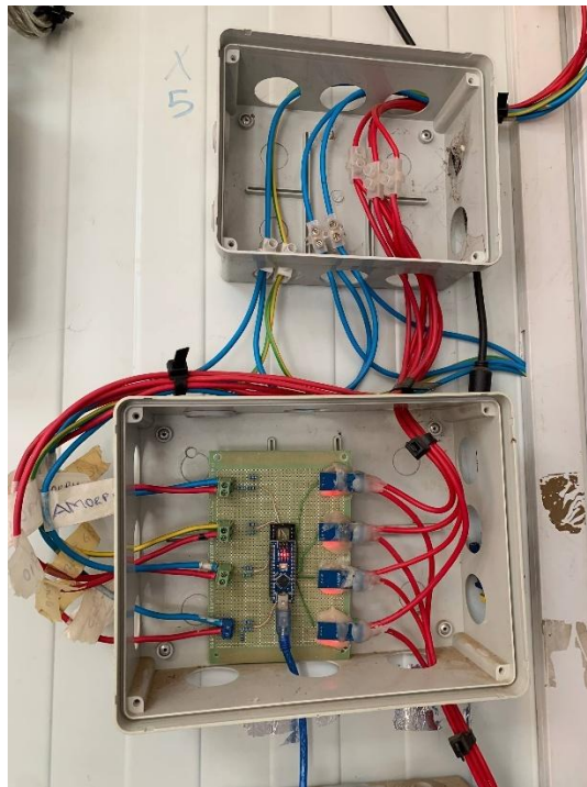
Figure 5.5 - Arduino Nano connection for measuring voltage and current.
