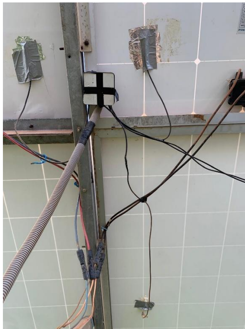
Figure 5.4 - Voltage sensor connected from the panels to the Arduino Nano.
