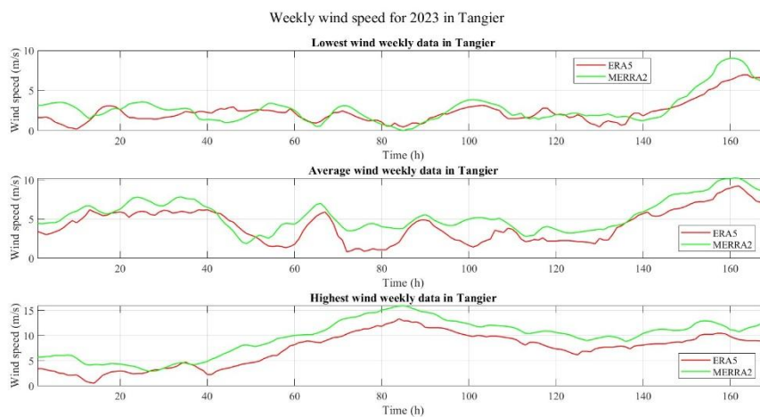
Figure 3.30 – Weekly wind speed profile in Tangier at 10 meters of height.
